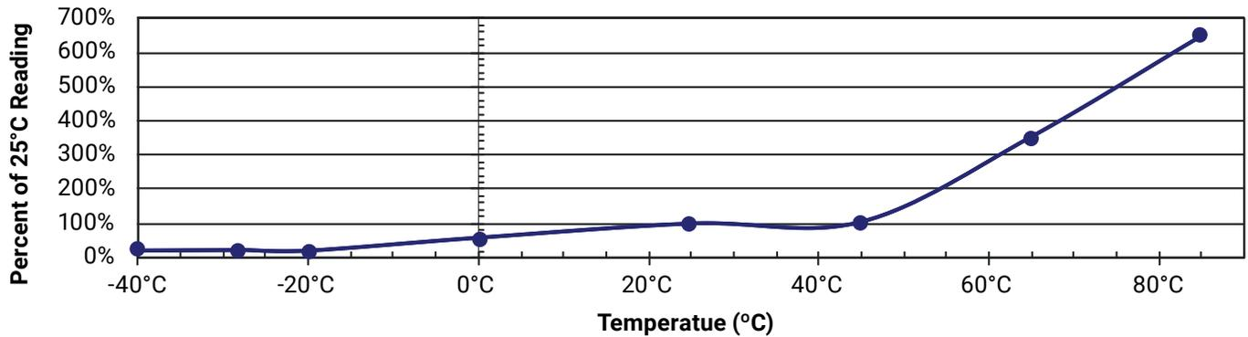
**EQUIVALENT SERIES RESISTANCE VS. TEMPERATURE**
