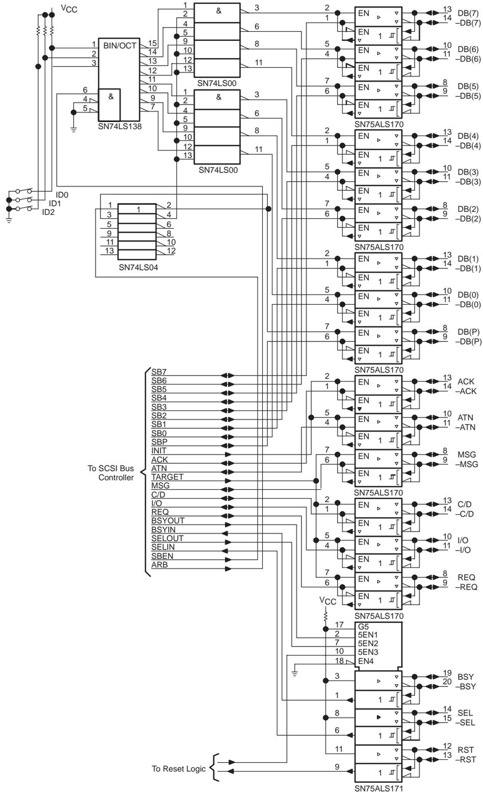
Figure 22. Typical Differential SCSI Bus Interface Implementation
