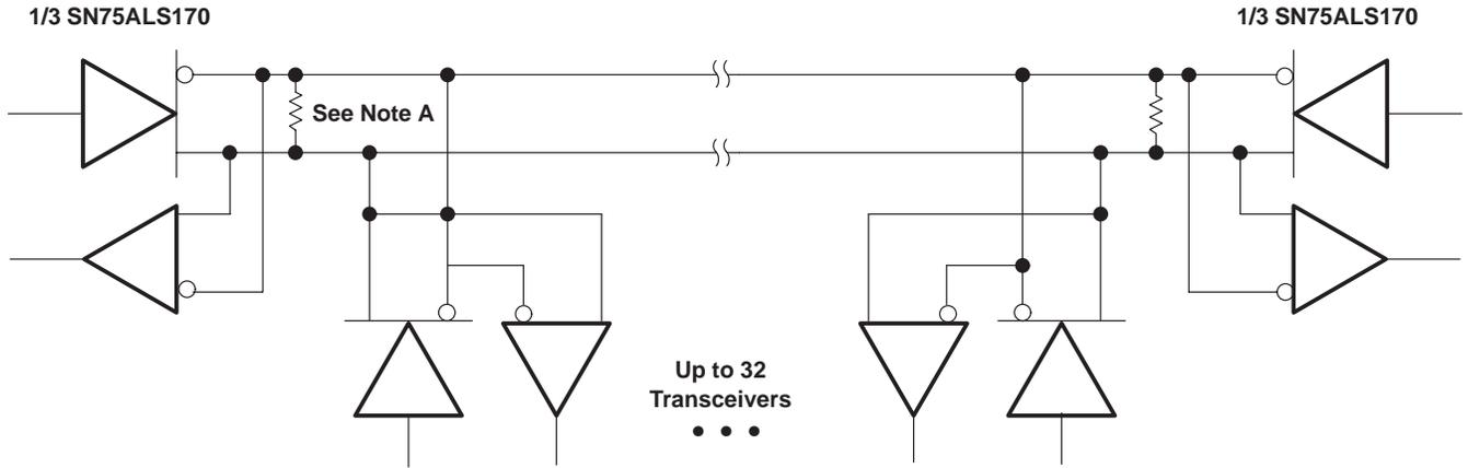
NOTE A: The line should be terminated at both ends in its characteristic impedance. Stub lengths off the main line should be kept as short as possible.
