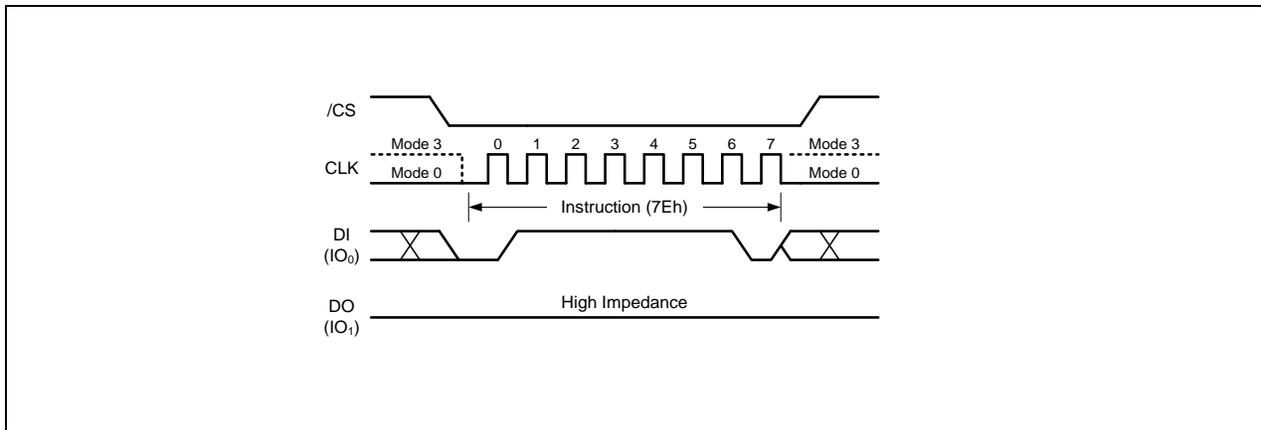
Figure 56. Global Block Lock Instruction for SPI Mode
