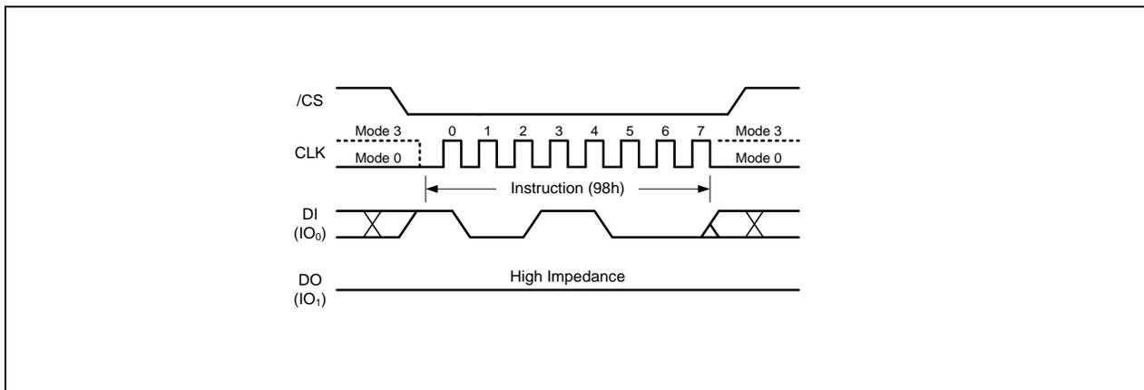
Figure 57. Global Block Unlock Instruction for SPI Mode
