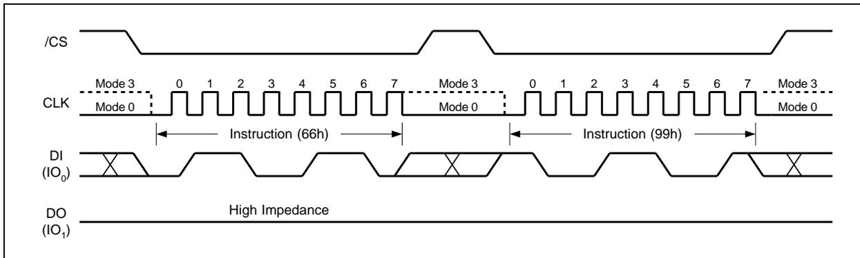
Figure 58a. Enable Reset and Reset Instruction Sequence
