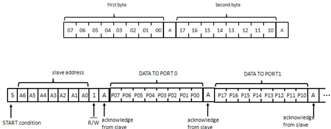
Figure 6: Correlation between bits and ports
