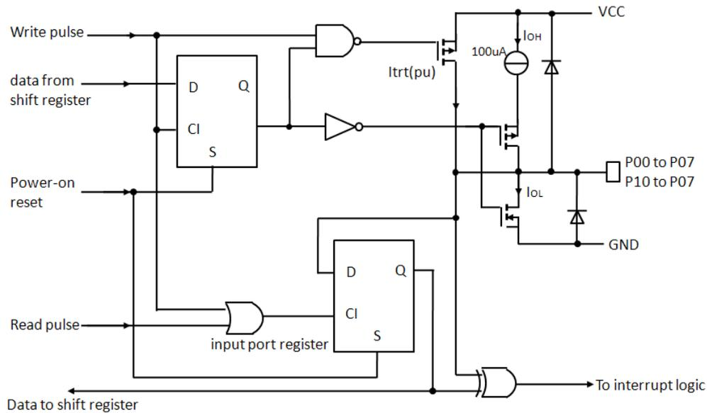
Figure 5: Simplified schematic diagram of P00 to P17
