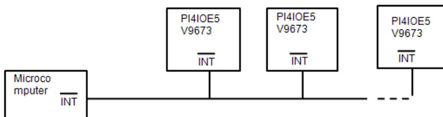
Figure 9: Application of multiple P4IOE5V9673s with interrupt
