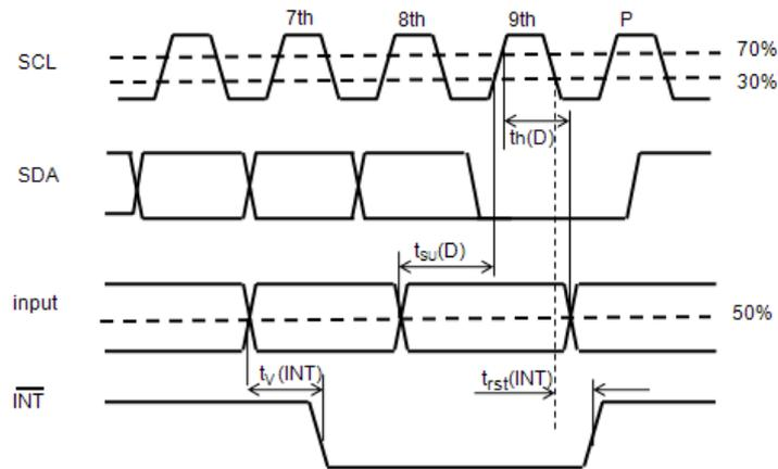
Figure 3: Timing Parameters for INT Signal
