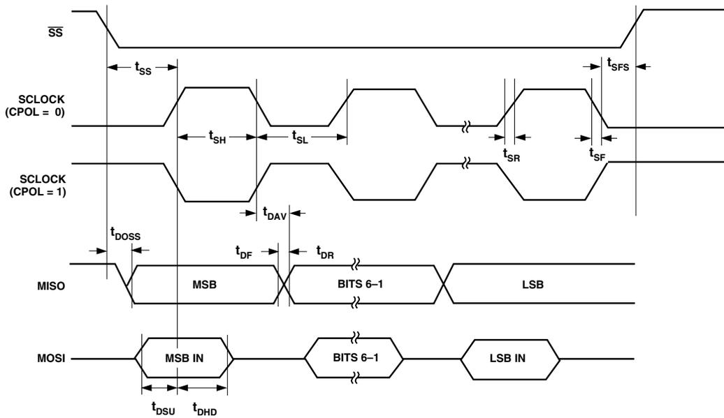
Figure 11. SPI Slave Mode Timing (CPHA = 0)
