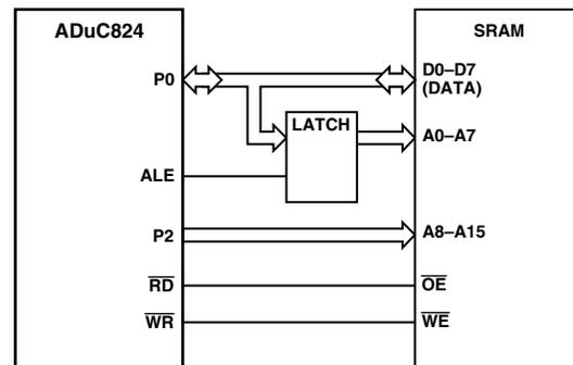
Figure 45. External Data Memory Interface (64 K Address Space)
