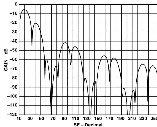
Figure 25. 60 Hz Normal Mode Rejection vs. SF
