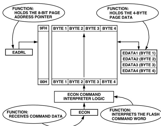
**Figure 31. Flash/EE Data Memory Control and Configuration**
