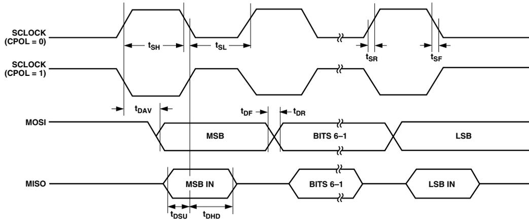
Figure 8. SPI Master Mode Timing (CPHA = 1)
