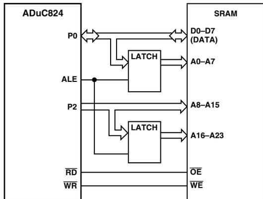
Figure 46. External Data Memory Interface (16 MBytes Address Space)
