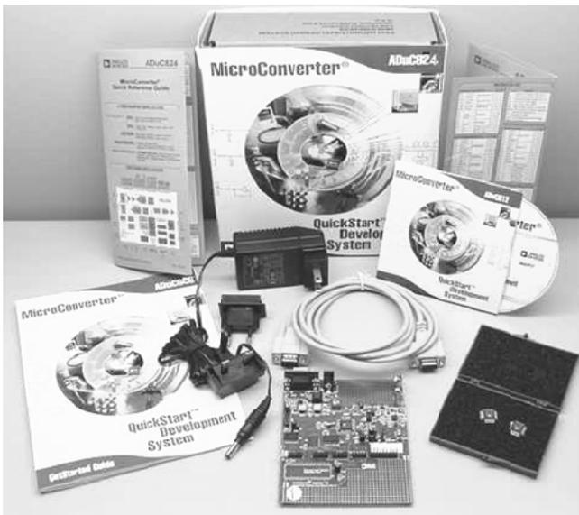
Figure 54. Components of the QuickStart Development System
