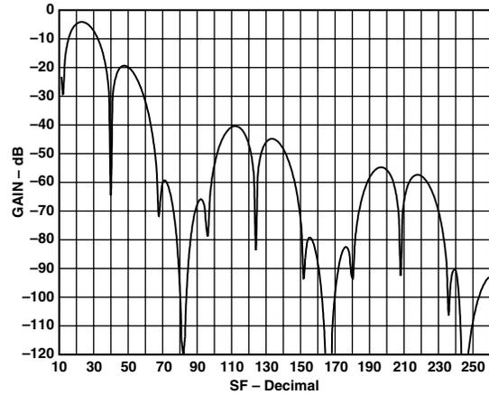
Figure 24. 50 Hz Normal Mode Rejection vs. SF
