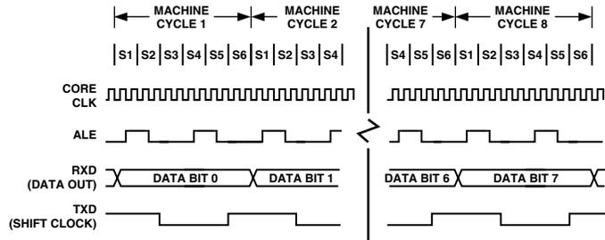
Figure 40. UART Serial Port Transmission, Mode 0.
