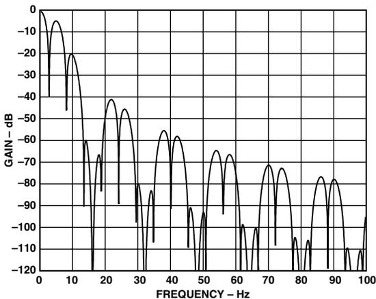
Figure 23. Filter Response, SF = 255 dec
