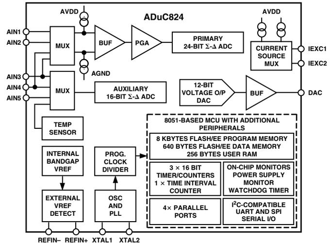
low-level signals). The ADCs with on-chip digital filtering are intended for the measurement of wide dynamic range, low-frequency signals, such as those in weigh scale, strain-gauge, pressure transducer, or temperature measurement applications. The ADC output data rates are programmable and the ADC output resolution will vary with the programmed gain and output rate.
