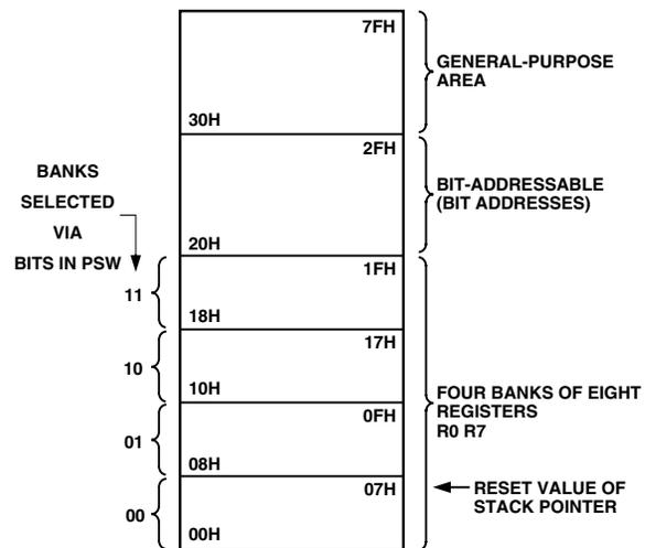
Figure 15. Lower 128 Bytes of Internal Data Memory
