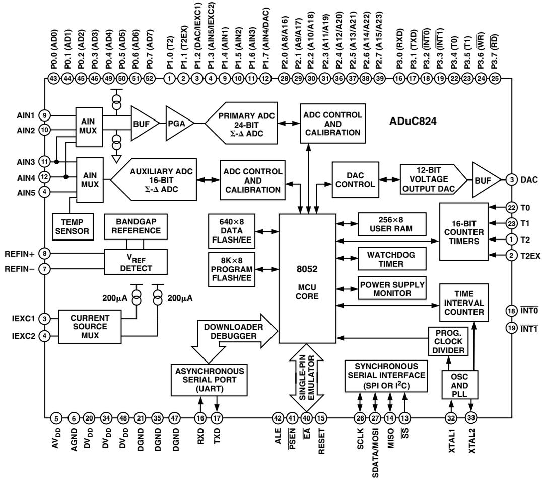
Figure 12. Block Diagram
