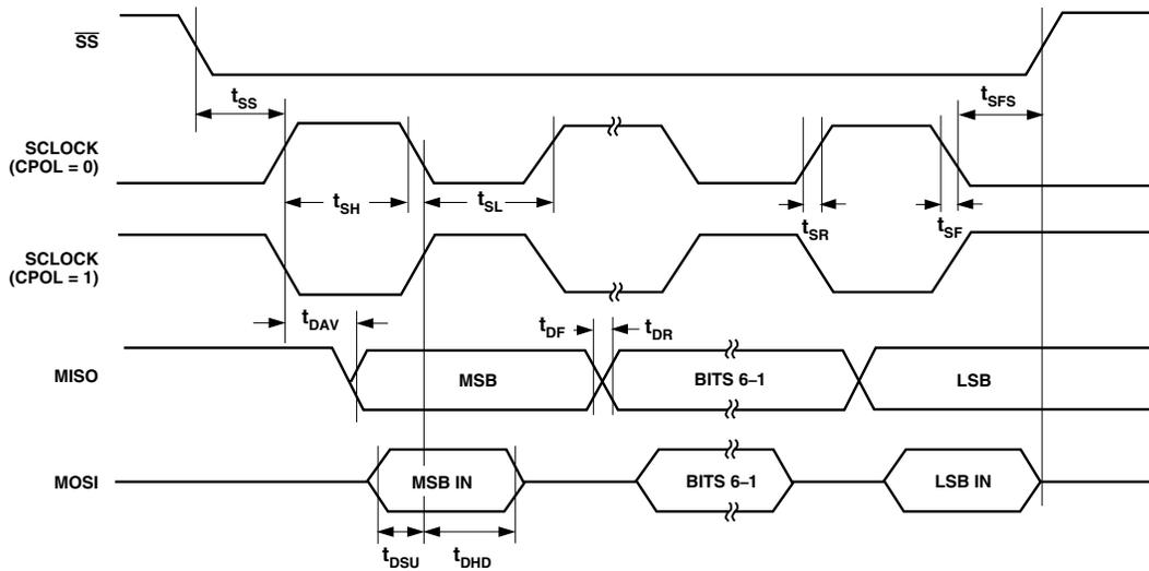
Figure 10. SPI Slave Mode Timing (CPHA = 1)
