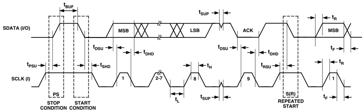
Figure 7. I<sup>2</sup>C-Compatible Interface Timing
