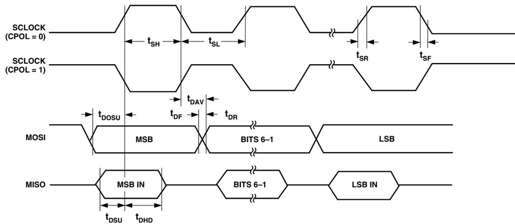
Figure 9. SPI Master Mode Timing (CPHA = 0)
