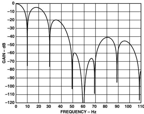
Figure 22. Filter Response, SF = 69 dec
