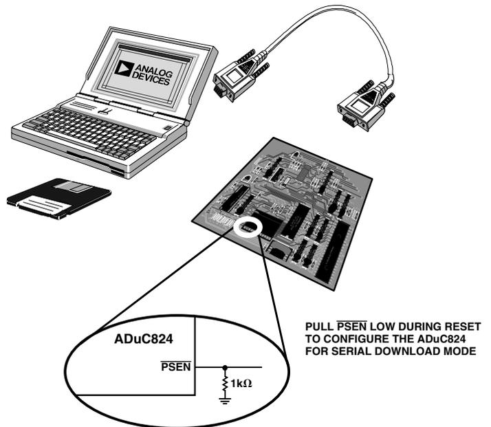
Figure 28. Flash/EE Memory Serial Download Mode Programming
