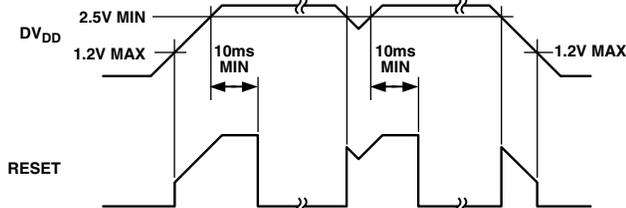
Figure 47. External POR Timing
