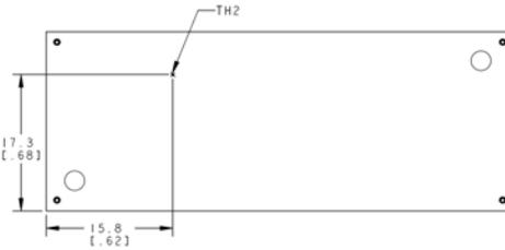
**Figure 19. Location of the thermal reference temperature TH<sub>2</sub> for Base Plate module. Do not exceed 110 °C.**
