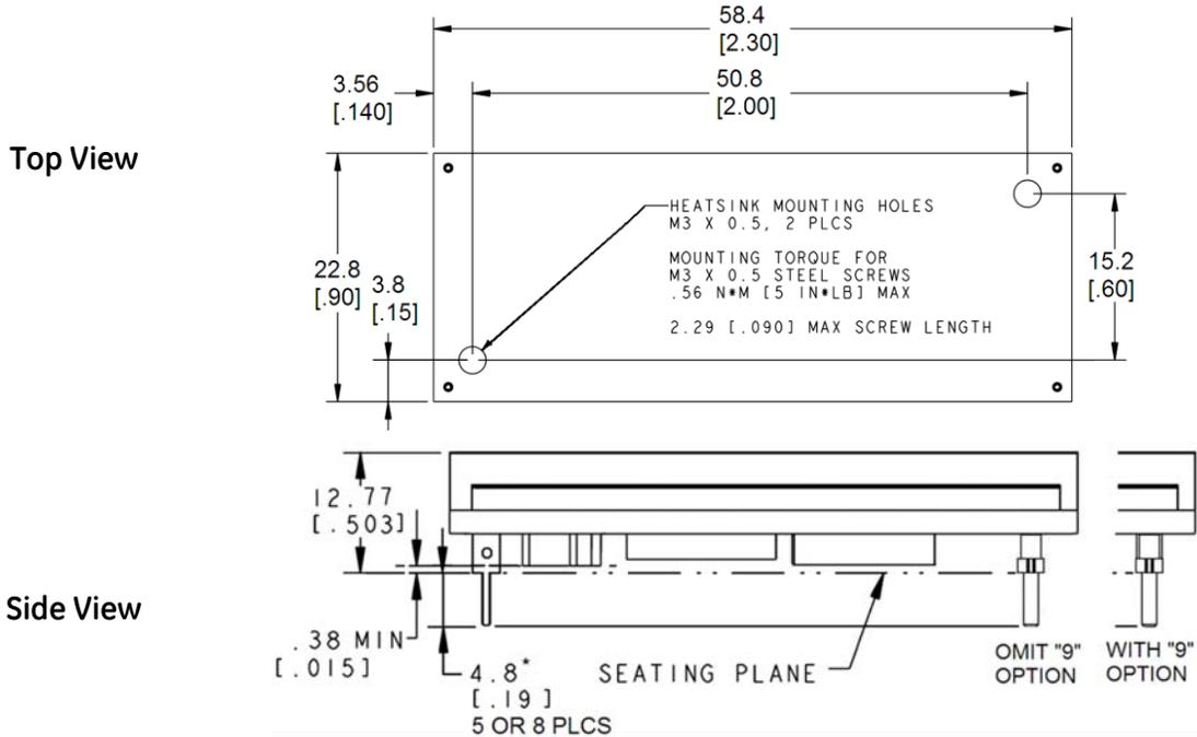
\*For optional pin lengths, see Table 2, Device Coding Scheme and Options
