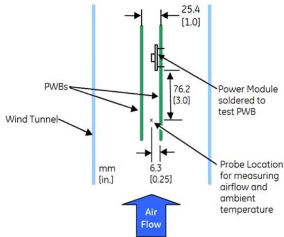
Heat-dissipating components are mounted on the top side of the module. Heat is removed by conduction, convection and radiation to the surrounding environment. Proper cooling can be verified by measuring the thermal reference temperature (TH<sub>x</sub>). Peak temperature (TH<sub>x</sub>) occurs at the position indicated in Figure 18 and 19. For reliable operation this temperature should not exceed the listed temperature threshold.
