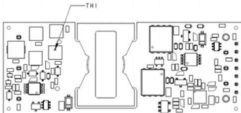
**Figure 18. Location of the thermal reference temperature TH<sub>1</sub>. Do not exceed 113 °C.**
