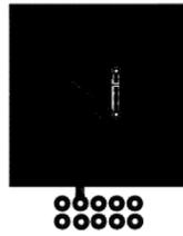
b. 55 °C/W when mounted on a 1 in<sup>2</sup> pad of 2 oz copper
