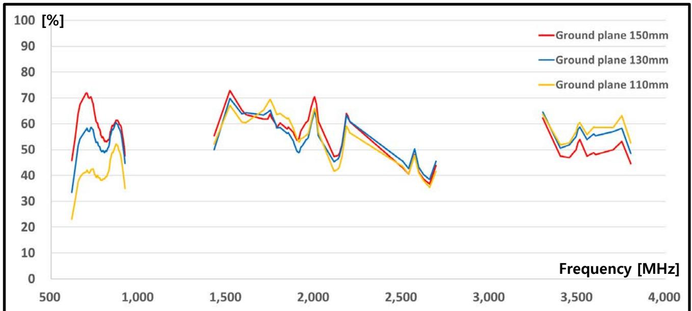
Data measured in free space and on reference ground plane of 150mm length and 45mm width, application data might vary
