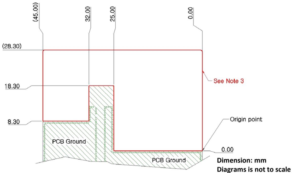
**NOTES: 1. Antenna must be mounted on the edge of PCB.**
