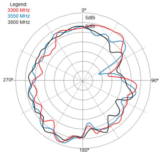
Data measured in free space and on reference ground plane of 150mm length and 45mm width, application data might vary
