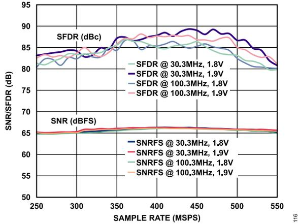
Figure 16. SNR/SFDR vs. Sample Rate and Supply
