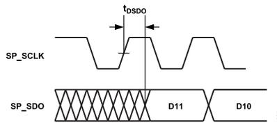
Figure 5. SP\_SDO Propagation Delay
