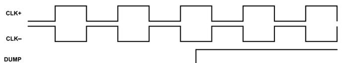
Figure 38. FIFO DUMP Timing
