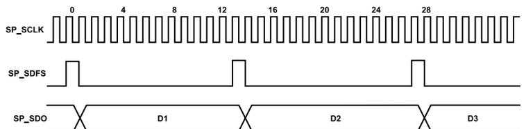
Figure 41. Data Output in Serial Bus Leader Mode
