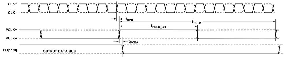
Figure 3. Parallel CMOS Mode Output Interface Timing
