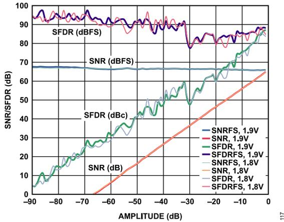
Figure 17. SNR/SFDR vs. Input Amplitude; 500 MSPS, 140.3 MHz
