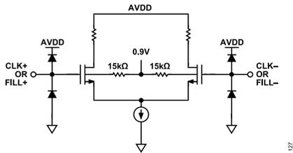
Figure 28. Equivalent CLK± and FILL± Input Circuit
