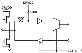
Figure 33. Equivalent SDIO Circuit
