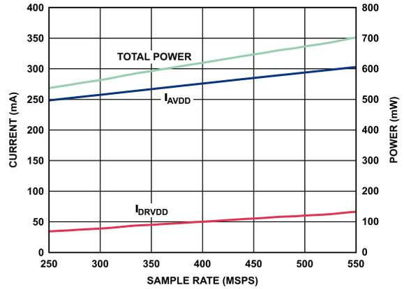
Figure 25. Current and Power vs. Sample Rate
