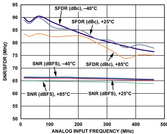
Figure 15. Single-Tone SNR/SFDR vs. Input Frequency ( $f_{IN}$ ) and Temperature; 500 MSPS
