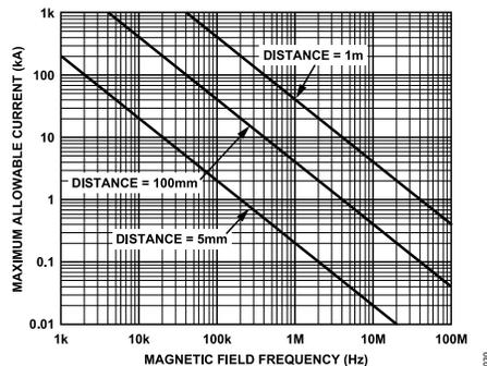
Figure 26. Maximum Allowable Current for Various Current-to-ADuM4135 Spacings
