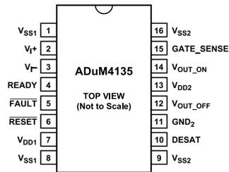
Figure 3. Pin Configuration
