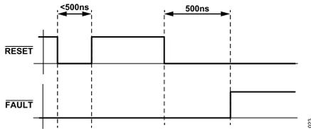
Figure 23. RESET Timing
