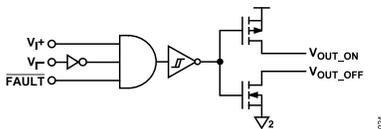
Figure 24. V<sub>I+</sub> and V<sub>I-</sub> Block Diagram
