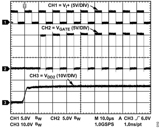
Figure 10. Typical  $V_{DD2}$  Startup to Output Valid
