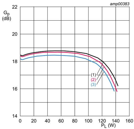
$V_{DS} = 28\text{ V}; I_{Dq} = 700\text{ mA}; t_p = 100\text{ }\mu\text{s}; \delta = 10\text{ \%}$ .
