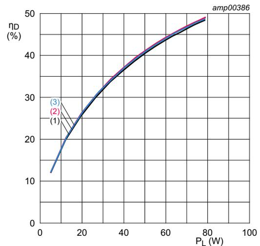
$V_{DS} = 28\text{ V}; I_{Dq} = 700\text{ mA.}$
