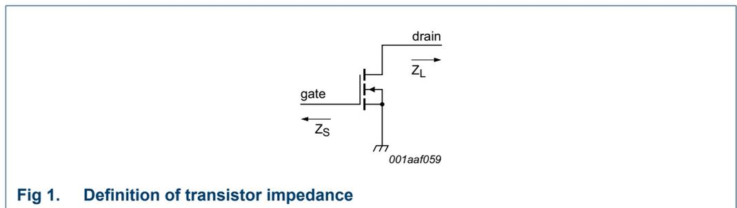
**Fig 1. Definition of transistor impedance**
