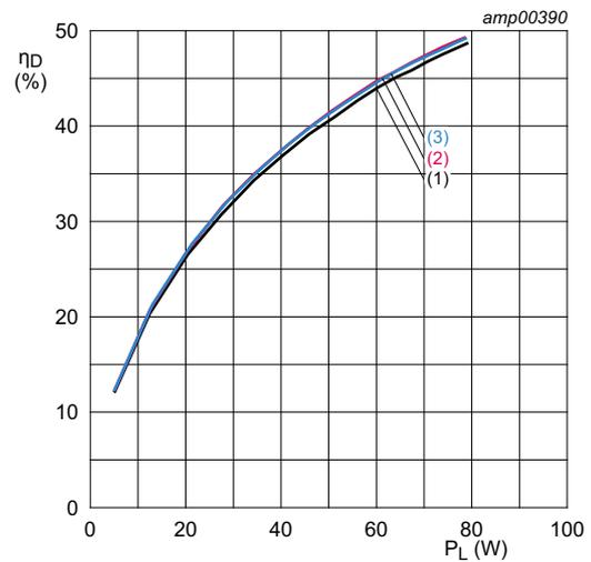
$V_{DS} = 28\text{ V}; I_{Dq} = 700\text{ mA}; 5\text{ MHz spacing}$
