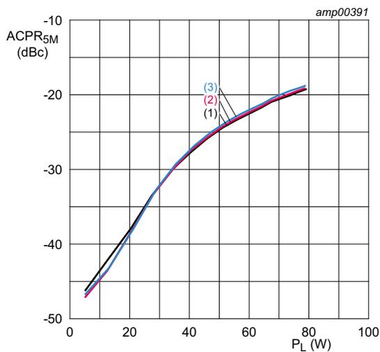
$V_{DS} = 28\text{ V}; I_{Dq} = 700\text{ mA}; 5\text{ MHz spacing}$
