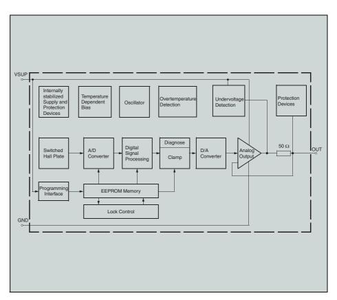
Fig. 2: Block diagram of the HAL 1880
