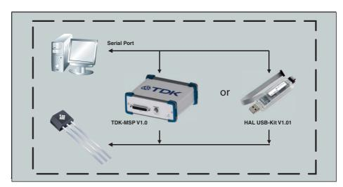
Fig. 1: Development tool setup
