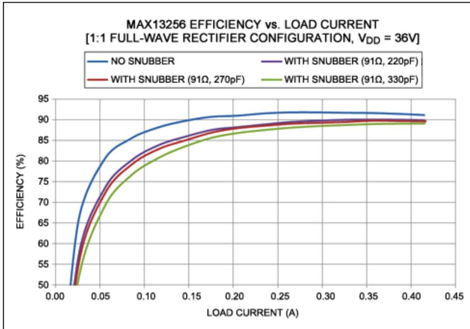
Figure 4. Efficiency vs. load measurements for the MAX13256.
