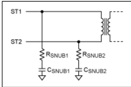
Figure 2. Simple RC snubbers for the MAX13256.
