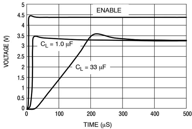
**Figure 15. Enable Transient**
