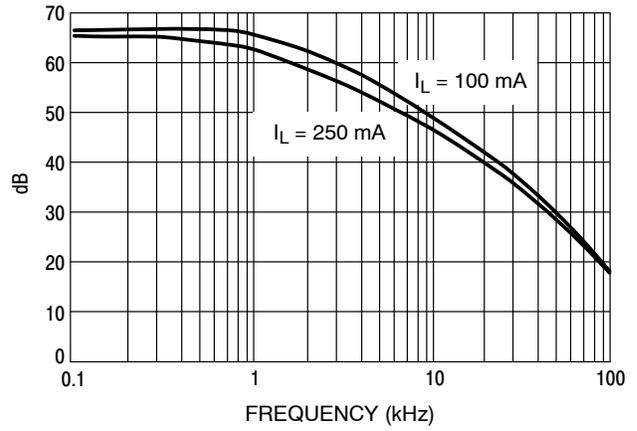
**Figure 14. Ripple Rejection**
