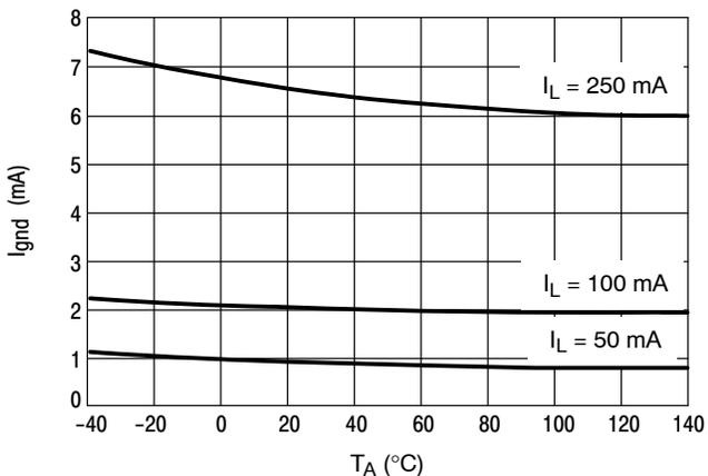
Figure 10. Ground Pin Current versus Ambient Temperature
