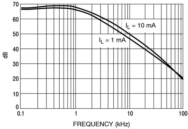
**Figure 13. Ripple Rejection**
