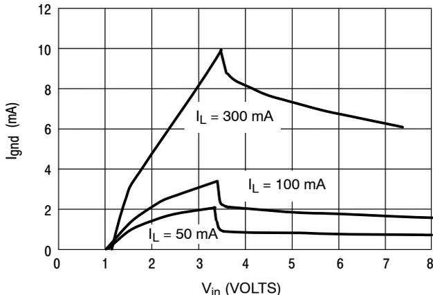
Figure 9. Ground Pin Current versus Input Voltage
