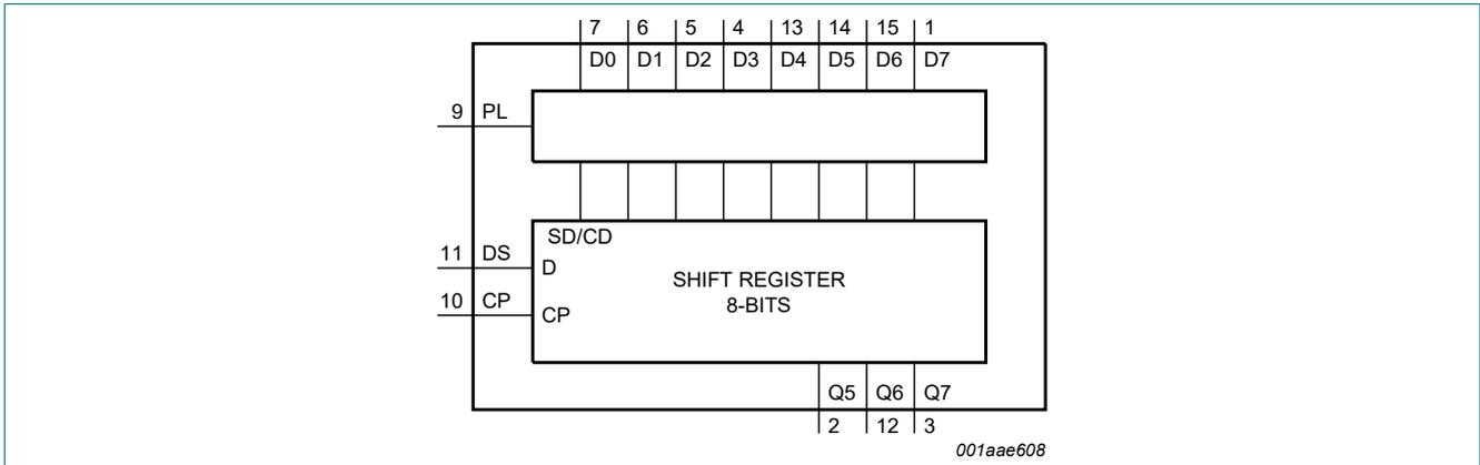
Fig. 1. Functional diagram
