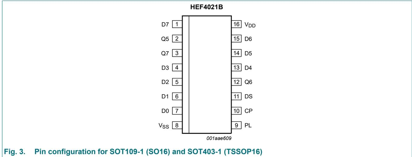
Fig. 3. Pin configuration for SOT109-1 (SO16) and SOT403-1 (TSSOP16)
