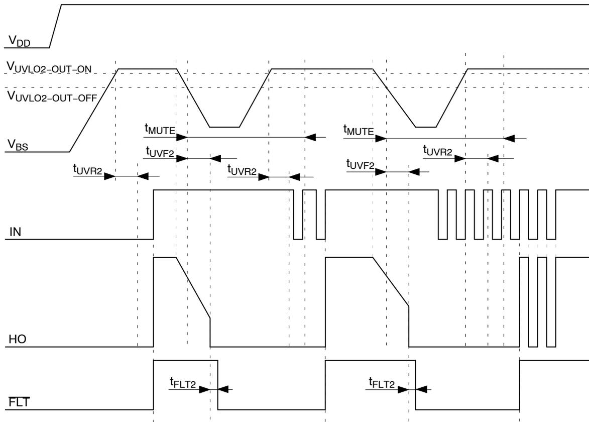
Figure 5. UVLO2 Waveform
