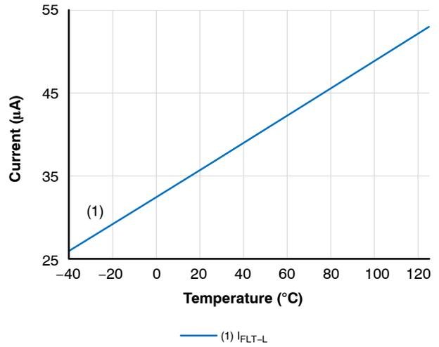
(Note: FLT = LOW,  $V_{DD} = 5$  V)
