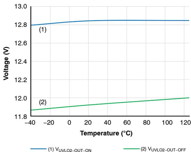
Figure 23. UVLO2 Threshold Voltage
