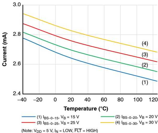
Figure 12.  $I_{BS}$  Supply Current,  $V_{DD} = 5$  V
