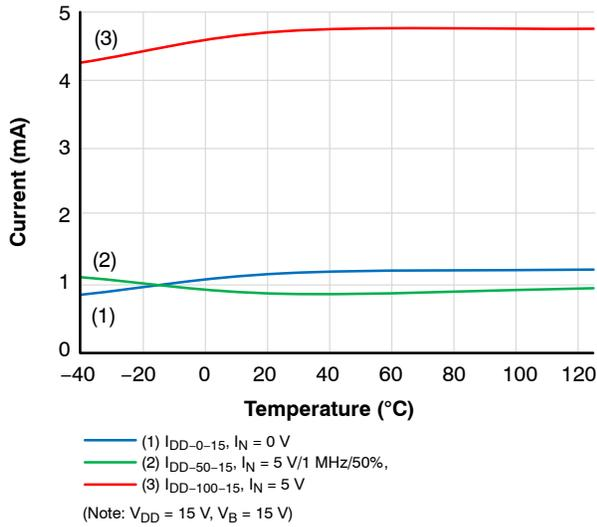
Figure 10.  $I_{DD}$  Supply Current,  $V_{DD} = 15$  V
