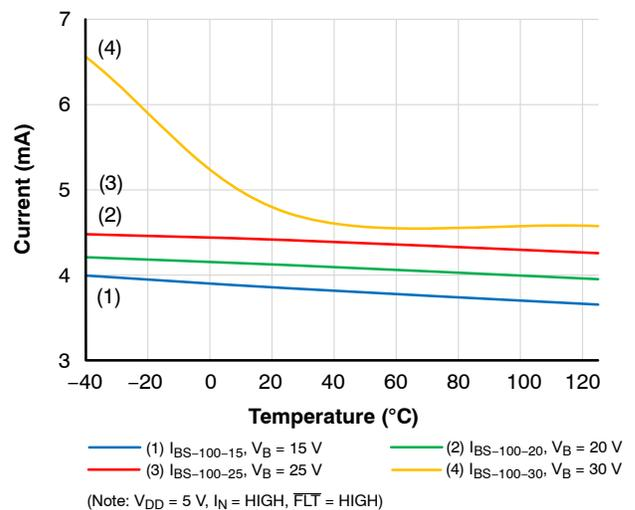
Figure 13.  $I_{BS}$  Supply Current,  $V_{DD} = 5$  V
