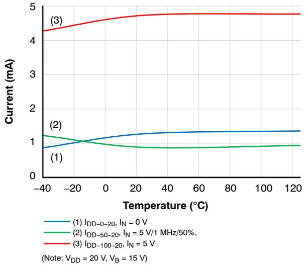
Figure 11.  $I_{DD}$  Supply Current,  $V_{DD} = 20$  V
