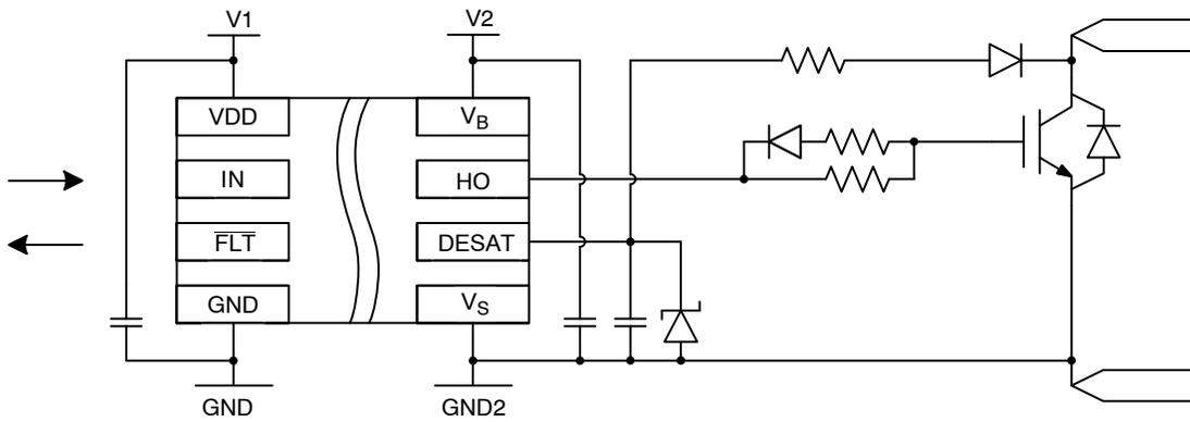
Figure 2. Simplified Application Schematics
