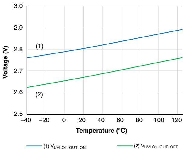
Figure 22. UVLO1 Threshold Voltage
