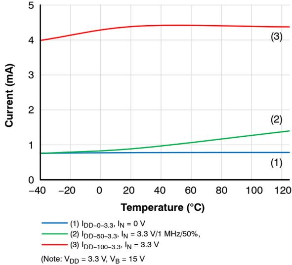
Figure 8.  $I_{DD}$  Supply Current,  $V_{DD} = 3.3$  V
