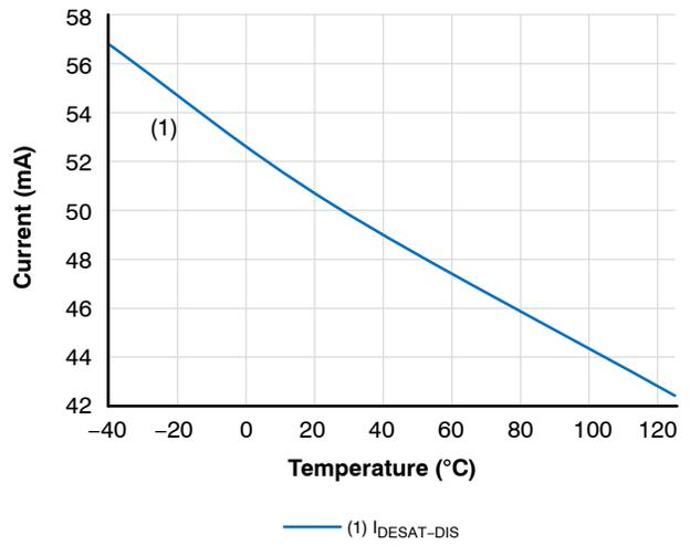
Figure 27. DESAT Blanking Discharge Current
