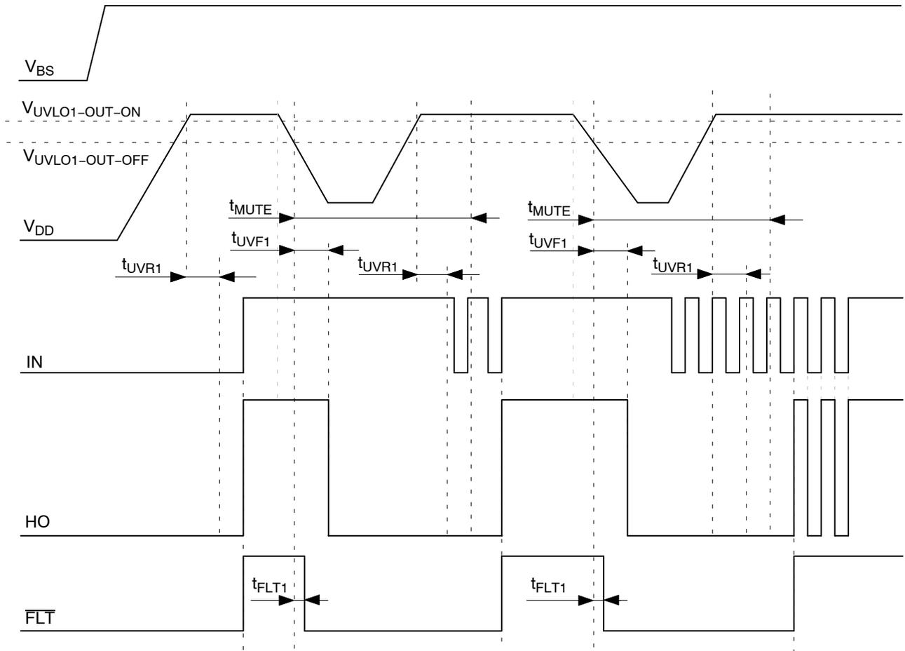
Figure 4. UVLO1 Waveform
