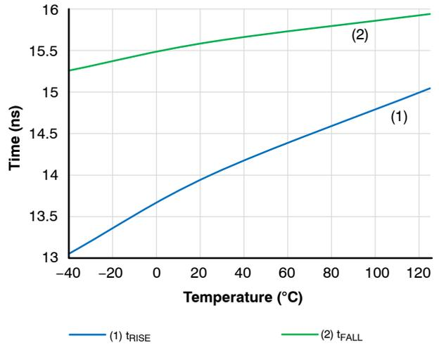
(Note:  $C_{LOAD} = 1\text{ nF}$ ,  $V_{BS} = 15\text{ V}$ )
