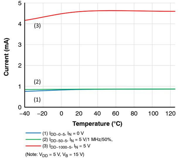
Figure 9.  $I_{DD}$  Supply Current,  $V_{BS} = 5$  V
