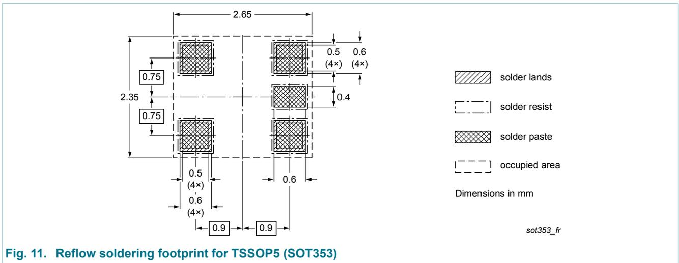
Fig. 11. Reflow soldering footprint for TSSOP5 (SOT353)
