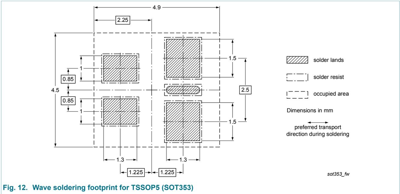
Fig. 12. Wave soldering footprint for TSSOP5 (SOT353)
