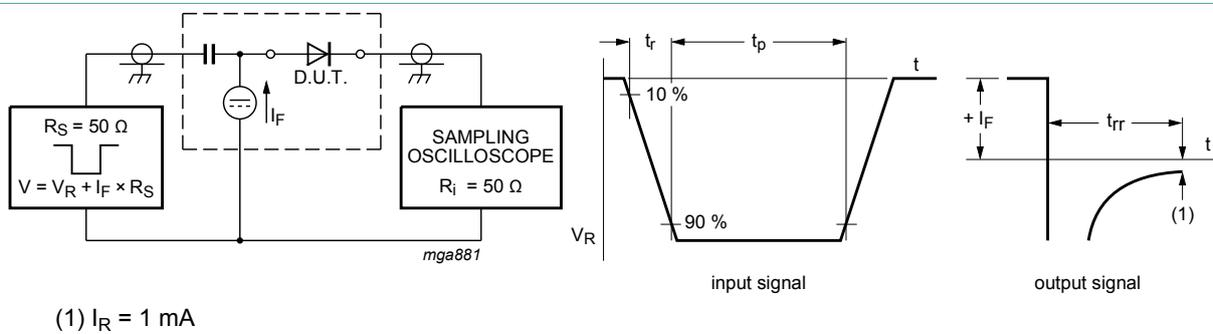
Fig. 8. Reverse recovery time: test circuit and waveforms
