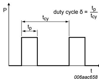
Fig. 9. Duty cycle definition
