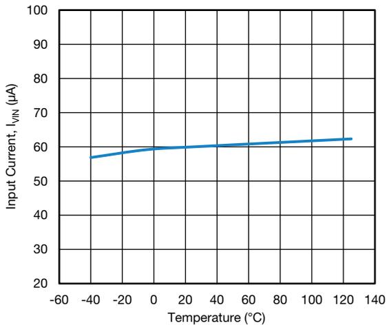
**Fig. 18 - Input Current vs. Junction Temperature**
