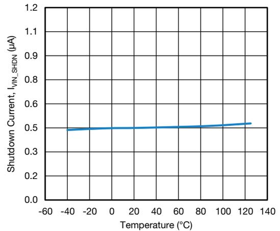
**Fig. 20 - Shutdown Current vs. Junction Temperature**
