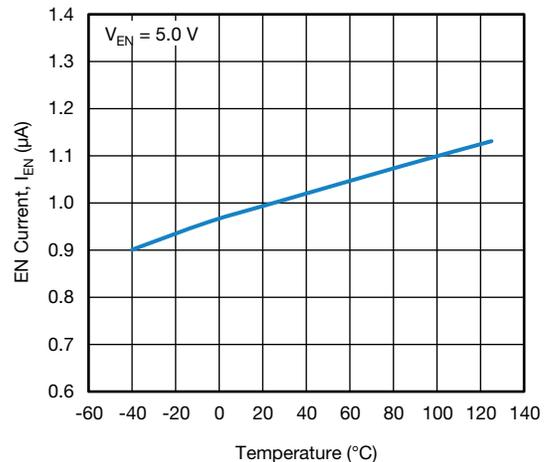
**Fig. 15 - EN Current vs. Junction Temperature**
