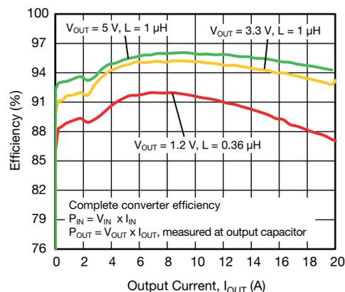
Fig. 2 - Efficiency vs. Output Current
