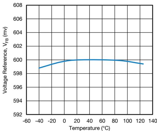
**Fig. 12 - Voltage Reference vs. Junction Temperature**
