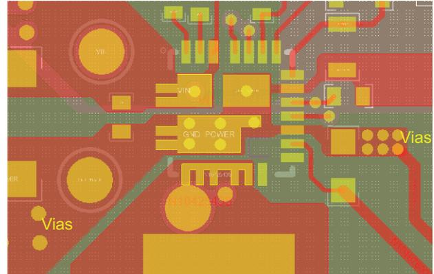
1. In order to minimize the ground voltage drop due to high current, it is recommended to place vias on the  $P_{GND}$  planes. Make use of the inner ground layers to lower the impedance
