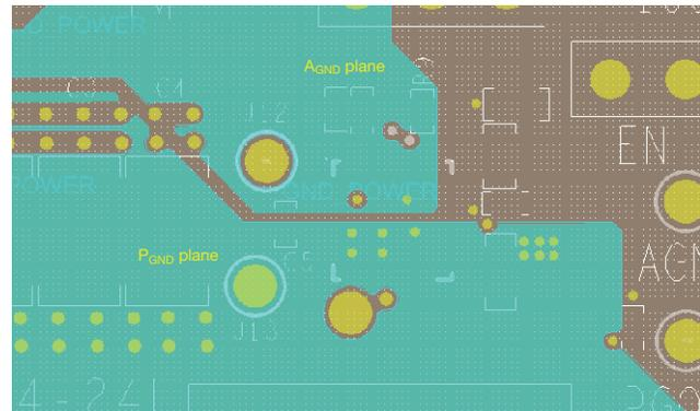
1. It is recommended to make the whole inner 1 layer (next to top layer) ground plane
