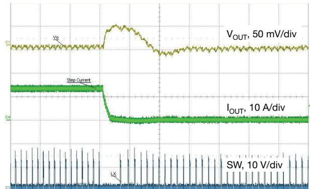
**Fig. 35 - Load Release, 12 A to 0.1 A, 1 A/ $\mu$ s,  $t = 20\text{ }\mu$ s/div
