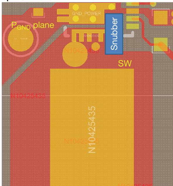
1. Connect output inductor to device with large plane to lower resistance
