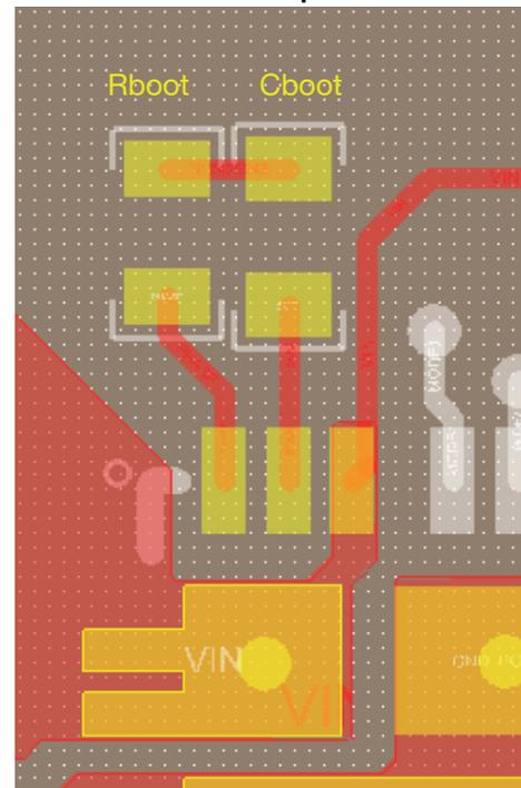
1.  $C_{BOOT}$  and  $R_{BOOT}$  need to be placed very close to the device, between PHASE and BOOT pins
