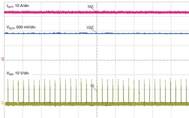
Fig. 26 - Overcurrent Protection Behavior,  $t = 5\text{ }\mu\text{s/div}$
