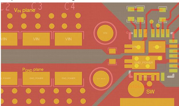
1. Thermal relief vias can be added to the  $V_{IN}$  and  $P_{GND}$  pads to utilize inner layers for high current and thermal dissipation
