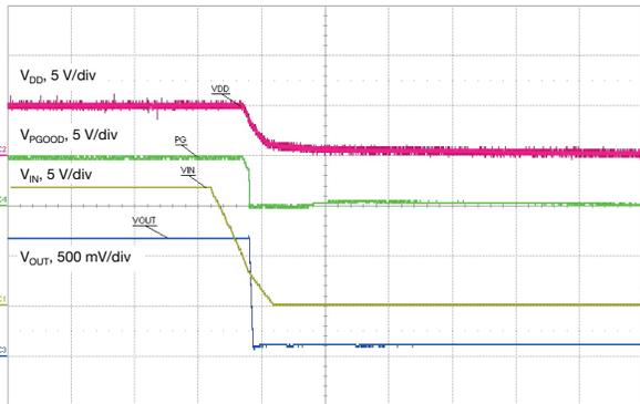
Fig. 25 - Shut down with  $V_{IN}$ ,  $t = 100\text{ ms/div}$
