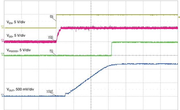
Fig. 27 - Startup with EN,  $t = 1\text{ ms/div}$
