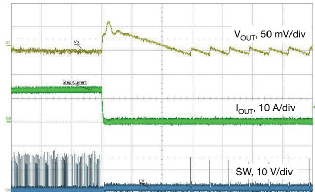
**Fig. 34 - Load Release, 12 A to 0.1 A, 1 A/ $\mu$ s,  $t = 50\text{ }\mu$ s/div
