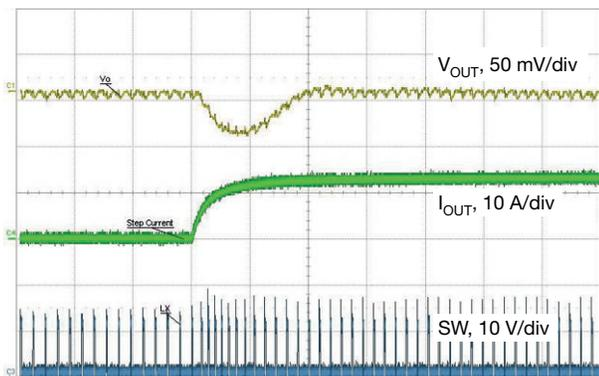
**Fig. 32 - Load Step, 0.1 A to 12 A, 1 A/ $\mu$ s,  $t = 10\text{ }\mu$ s/div
