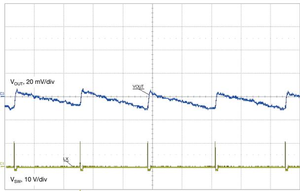
**Fig. 37 - Output Ripple, 0.1 A,  $t = 20\text{ }\mu\text{s/div}$
