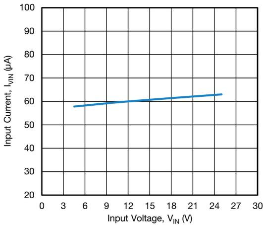
**Fig. 17 - Input Current vs. Input Voltage**
