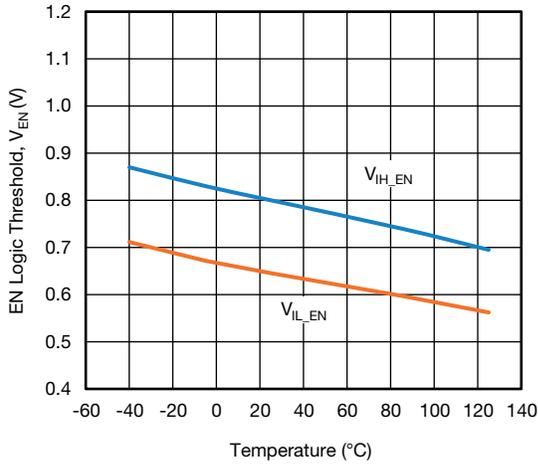
**Fig. 16 - EN Logic Threshold vs. Junction Temperature**
