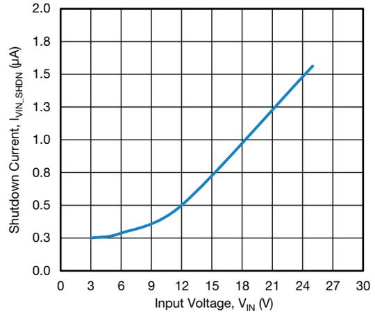
**Fig. 19 - Shutdown Current vs. Input Voltage**
