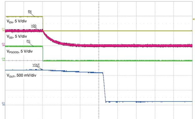
Fig. 28 - Shut down with EN,  $t = 200\text{ ms/div}$
