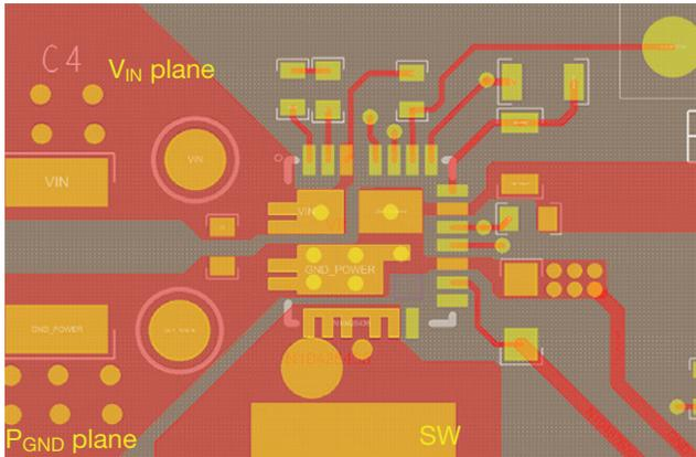
1. Layout  $V_{IN}$  and  $P_{GND}$  planes as shown above
