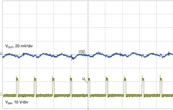
**Fig. 36 - Output Ripple, 0.1 A,  $t = 2\text{ }\mu\text{s/div}$
