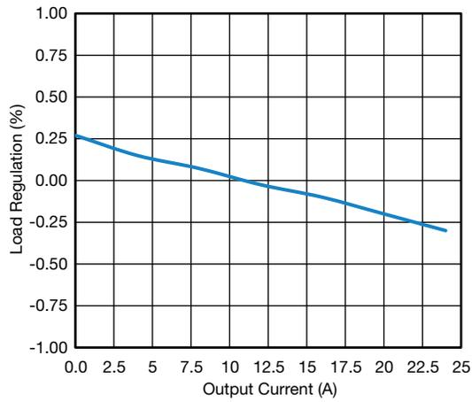
**Fig. 22 - Load Regulation vs. Output Current**
