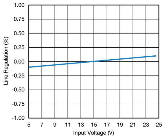
**Fig. 21 - Line Regulation vs. Input Voltage**
