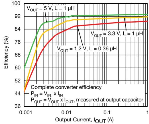
**Fig. 13 - Efficiency vs. Output Current**
