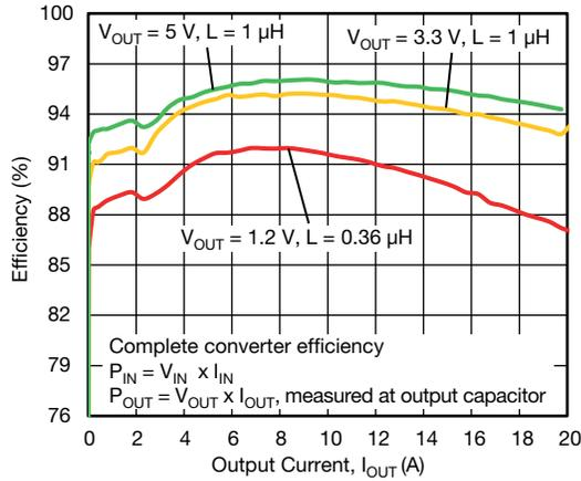
**Fig. 10 - Efficiency vs. Output Current**
