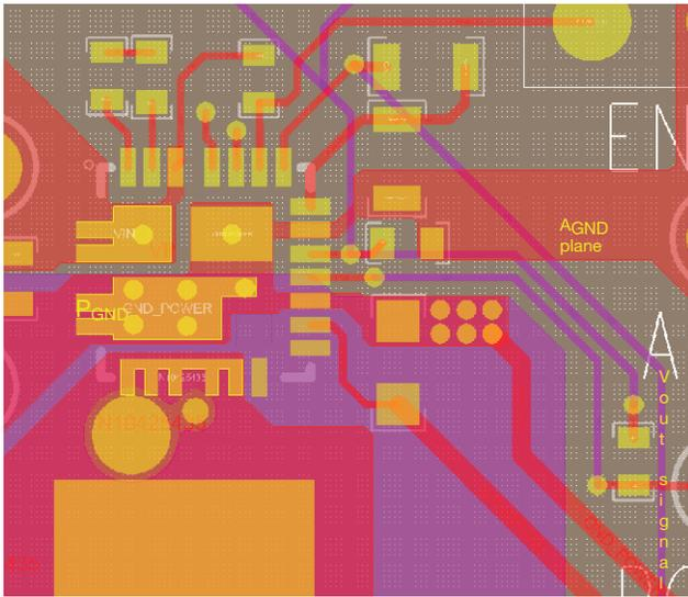
1. Separate the small analog signal from high current path. As shown above, the high paths with high  $dv/dt$ ,  $di/dt$  are placed on the left side of the IC, while the small control signals are placed on the right side of the IC. All the components for small analog signal should be placed closer to IC with minimum trace length
