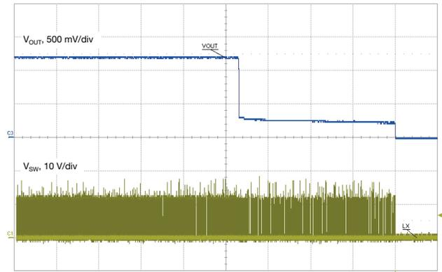
Fig. 29 - Output Undervoltage Protection Behavior,  $t = 50\text{ ms/div}$
