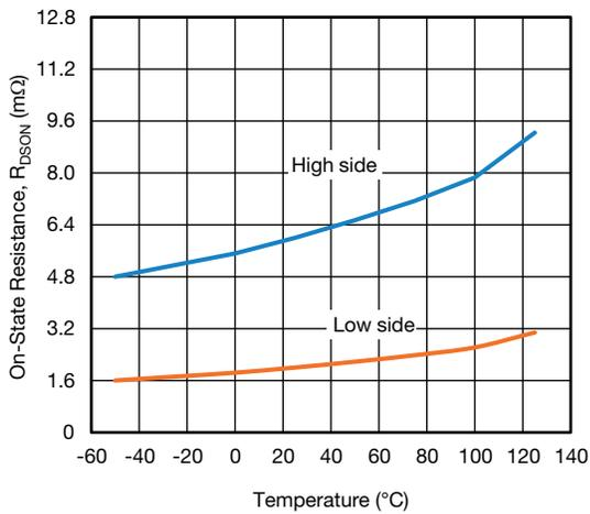
**Fig. 23 - On Resistance vs. Junction Temperature**
