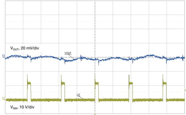
**Fig. 38 - Output Ripple, 12 A,  $t = 1\text{ }\mu\text{s/div}$
