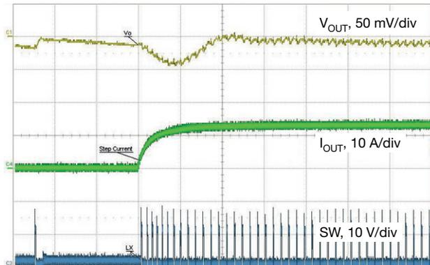
**Fig. 31 - Load Step, 0.1 A to 12 A, 1 A/ $\mu$ s,  $t = 10\text{ }\mu$ s/div
