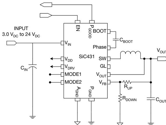
Fig. 1 - Typical Application Circuit for SiC431
