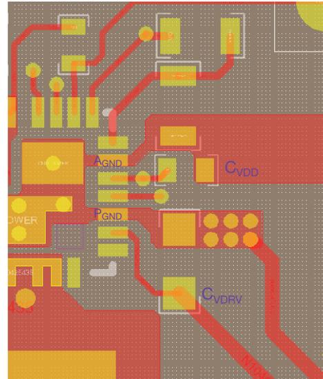
1.  $C_{VDD}$  cap should be placed between  $V_{DD}$  and  $A_{GND}$  to achieve best noise filtering
