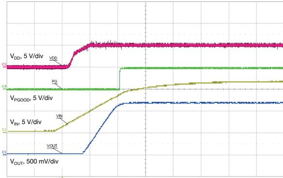
Fig. 24 - Startup with  $V_{IN}$ ,  $t = 2\text{ ms/div}$
