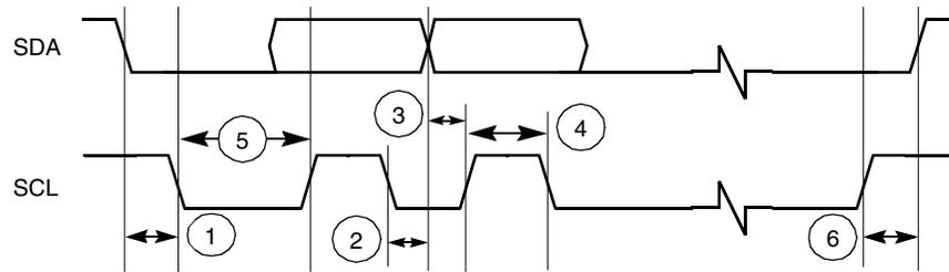
Figure 72. Definition of Bus Timing for I<sup>2</sup>C
