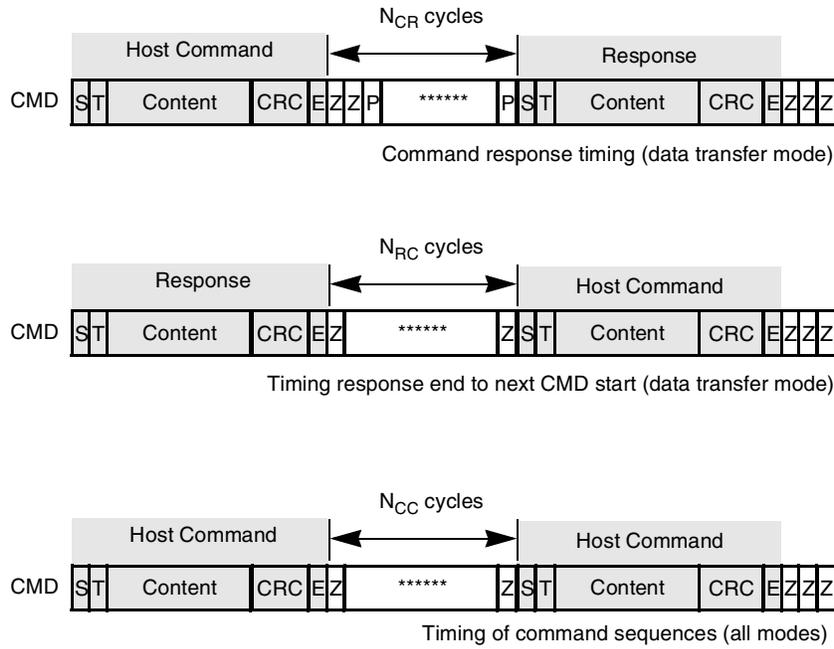
**Figure 19. Timing Diagrams at Data Transfer Mode**
