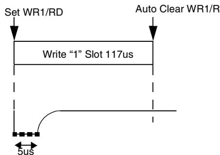
Figure 40. Write 1 Timing
