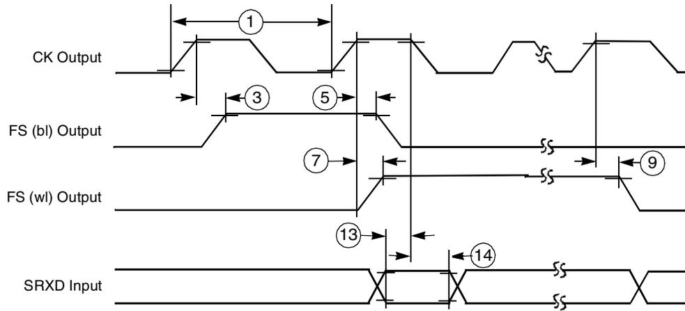
**Figure 35. SSI Receiver Internal Clock Timing Diagram**
