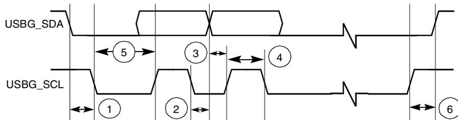
**Figure 44. USB Timing Diagram for Data Transfer from USB Transceiver (I<sup>2</sup>C)**
