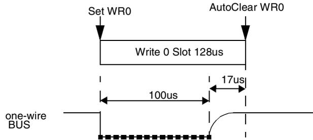
Figure 39. Write 0 Timing
