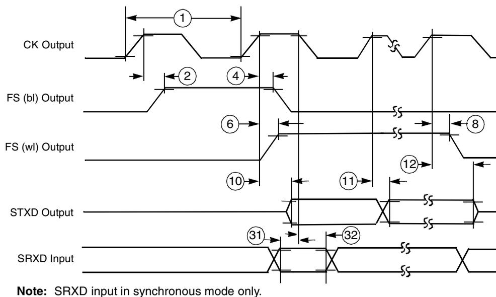
**Figure 34. SSI Transmitter Internal Clock Timing Diagram**
