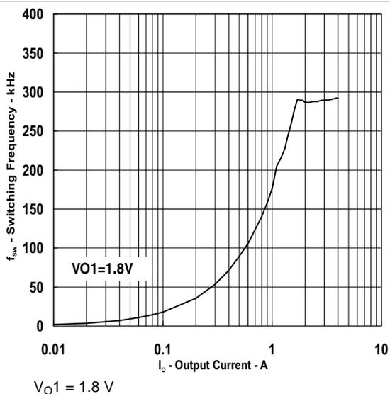
Figure 14. Switching Frequency vs Output Current (Ch1)
