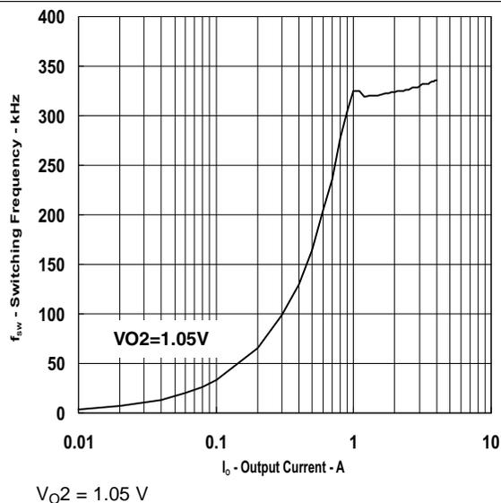
Figure 15. Switching Frequency vs Output Current (Ch2)
