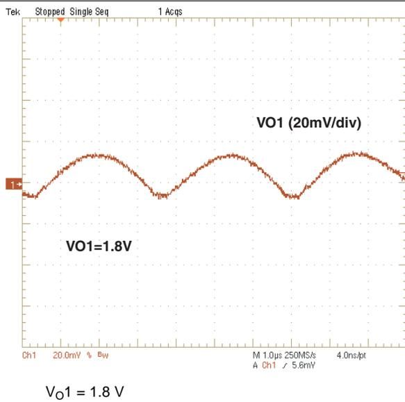
**Figure 26. 1.8-V Output Ripple Voltage**
