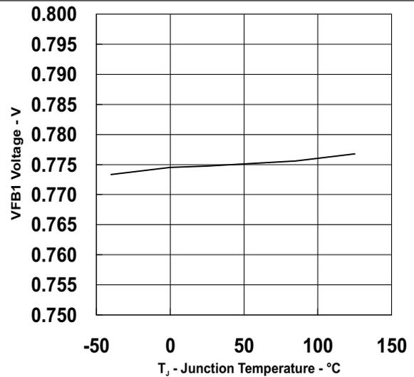
**Figure 8. VFB1 Voltage vs Junction Temperature**
