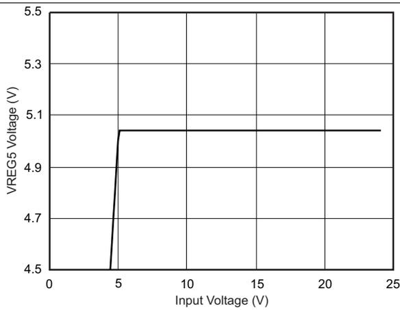
**Figure 5. VREG5 Voltage vs Input Voltage**
