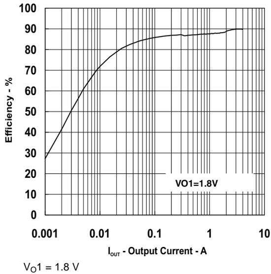
**Figure 24. 1.8-V Efficiency vs Output Current (Ch1)**
