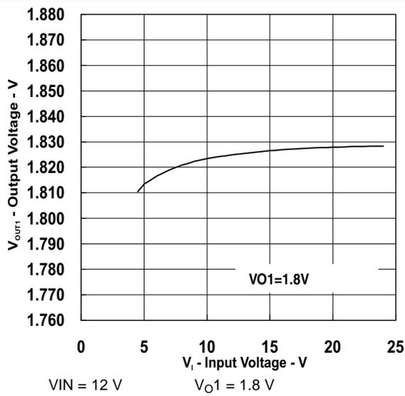
Figure 18. Output Voltage vs Input Voltage (Ch1)
