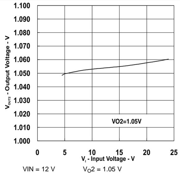
Figure 19. Output Voltage vs Input Voltage (Ch2)
