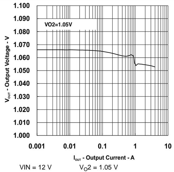
Figure 17. Output Voltage vs Output Current (Ch2)
