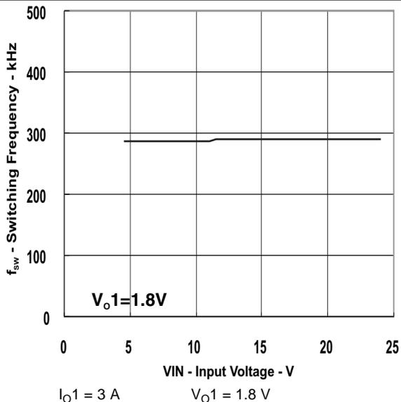
Figure 12. Switching Frequency vs Input Voltage (Ch1)
