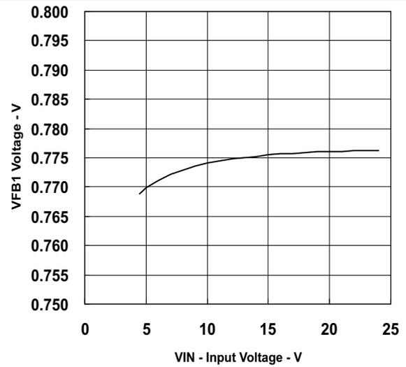
**Figure 6. VFB1 Voltage vs Input Voltage**
