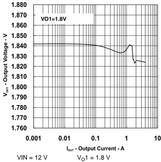
Figure 16. Output Voltage vs Output Current (Ch1)
