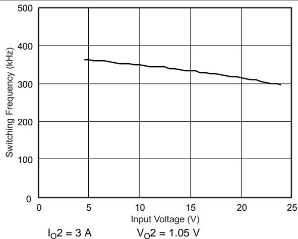
Figure 13. Switching Frequency vs Input Voltage (Ch2)
