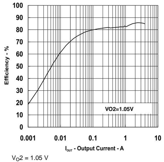
**Figure 25. 1.05-V Efficiency vs Output Current (Ch2)**
