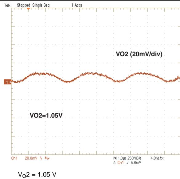
**Figure 27. 1.05-V Output Ripple Voltage**
