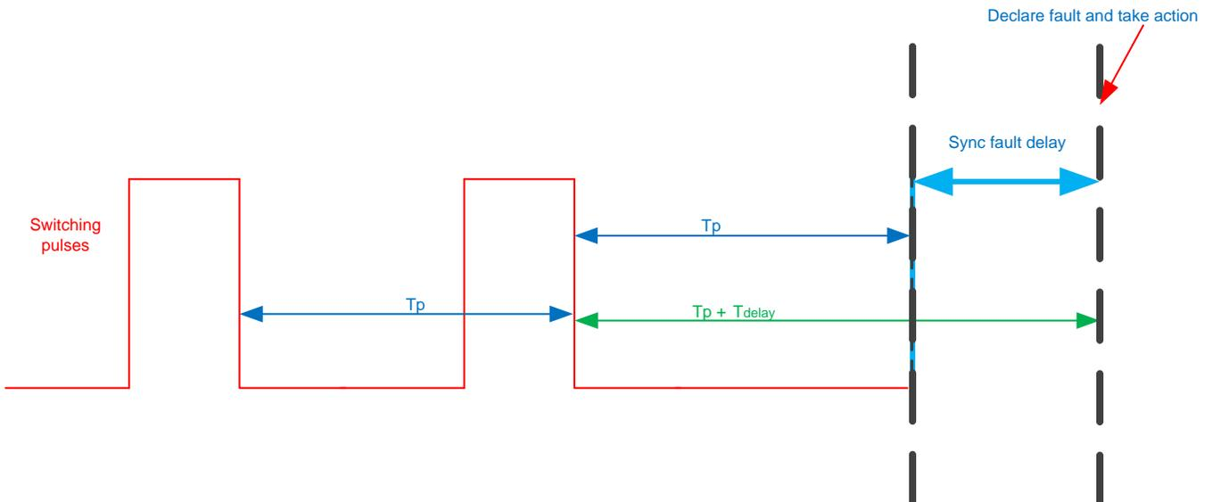
Figure 25. Switching Response When Sync Clock Lost
