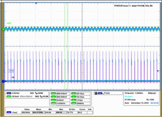
Figure 13. Output Voltage Ripple at Steady State
