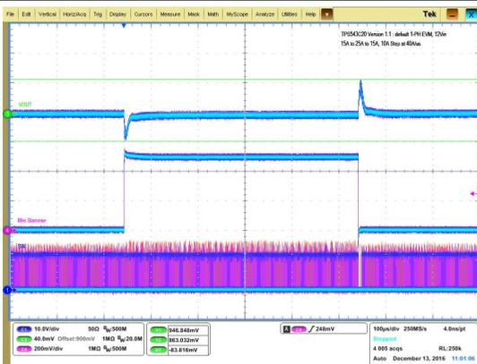
Figure 27. Transient Response of 0.9-V Output at 12-V<sub>IN</sub>, Transient is 15 A to 25 A to 15 A, the Step is 10 A at 40 A/μs
