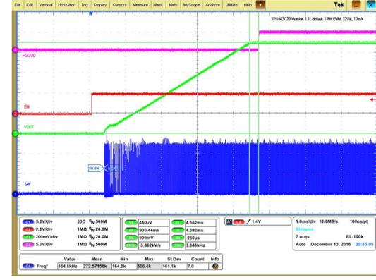
Figure 30. Start up from Control, 0.9-V Output at 12-V<sub>IN</sub>, 10-mA Output
