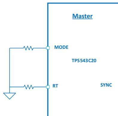
**Figure 16. Standalone: RT Pin Sets the Switching Frequency**
