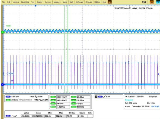
Figure 29. Output Ripple and SW Node of 0.9-V Output at 12-V<sub>IN</sub>, 0-A Output
