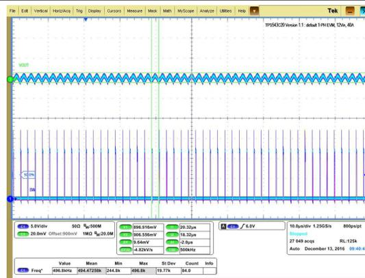
Figure 28. Output Ripple and SW Node of 0.9-V Output at 12-V<sub>IN</sub>, -A Output
