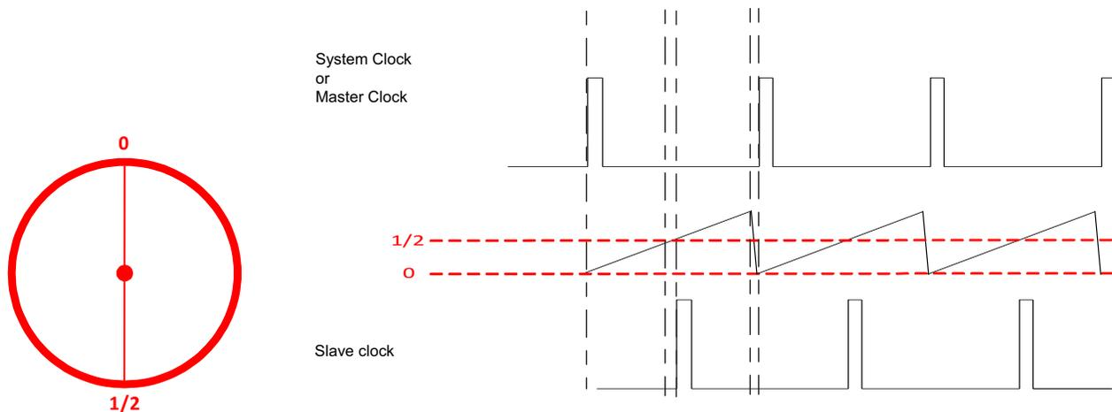
Figure 18. 2-Phase Stackable with 180° Clock Phase Shift
