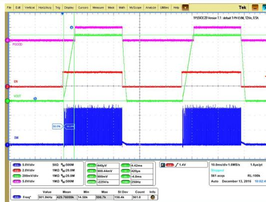
Figure 32. Output Voltage Start-up and Shutdown, 0.9-V Output at 12-V<sub>IN</sub>, 0.5-A Output
