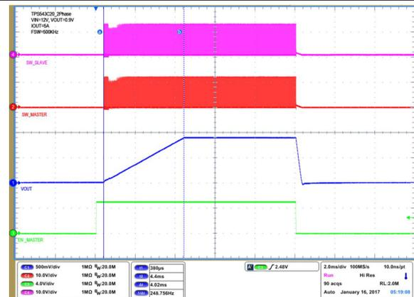
Figure 41. Output Voltage Start-up and Shutdown, 0.9-V Output at 12 V<sub>IN</sub>, 5-A Output
