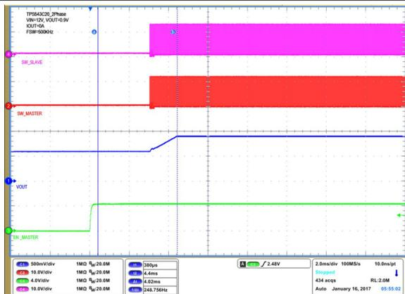
Figure 40. 0.6-V Pre-Bias Start Up From Enable, 0.9-V Output at 12 V<sub>IN</sub>, 0-A Output
