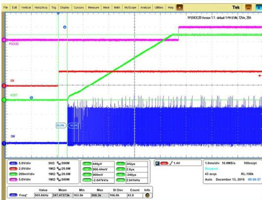
Figure 31. 0.5-V Prebias start up from Control, 0.9-V Output at 12-V<sub>IN</sub>, 20-A Output
