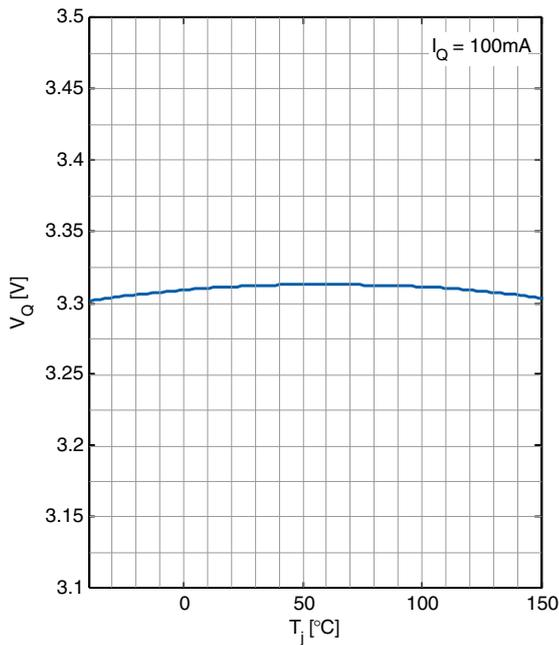
Output Voltage  $V_Q$  versus Junction Temperature  $T_j$  (5 V version)
