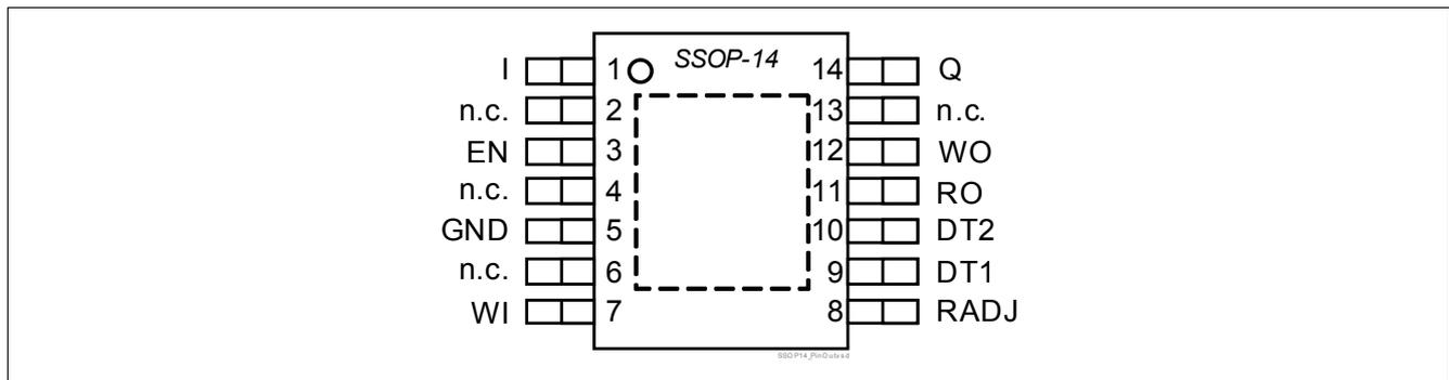
Figure 3 Pin Configuration
