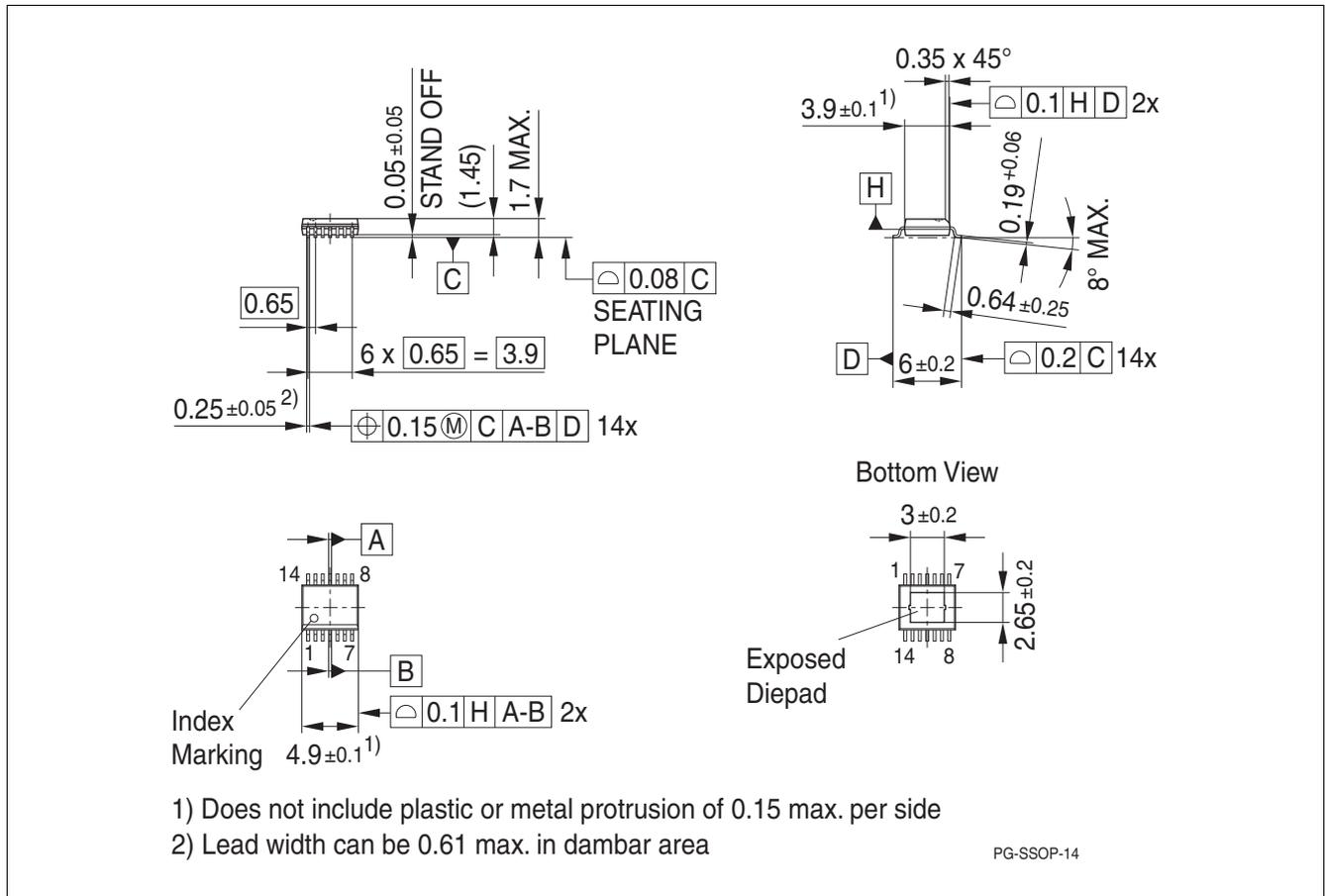
Figure 14 PG-SSOP-14
