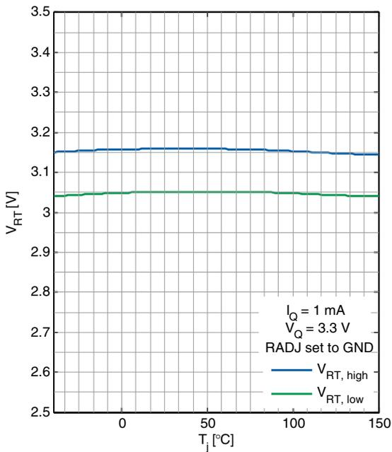
Undervoltage Reset Threshold  $V_{RT}$  versus Junction Temperature  $T_j$  (5 V version)
