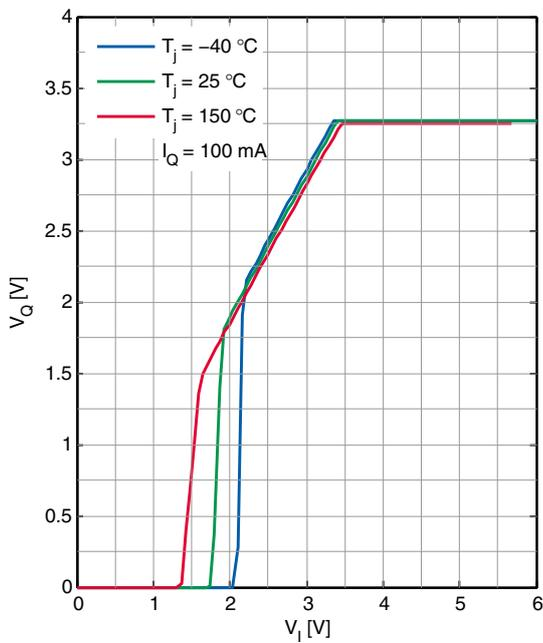
**Output Voltage  $V_Q$  versus Input Voltage  $V_I$  (5 V version)**
