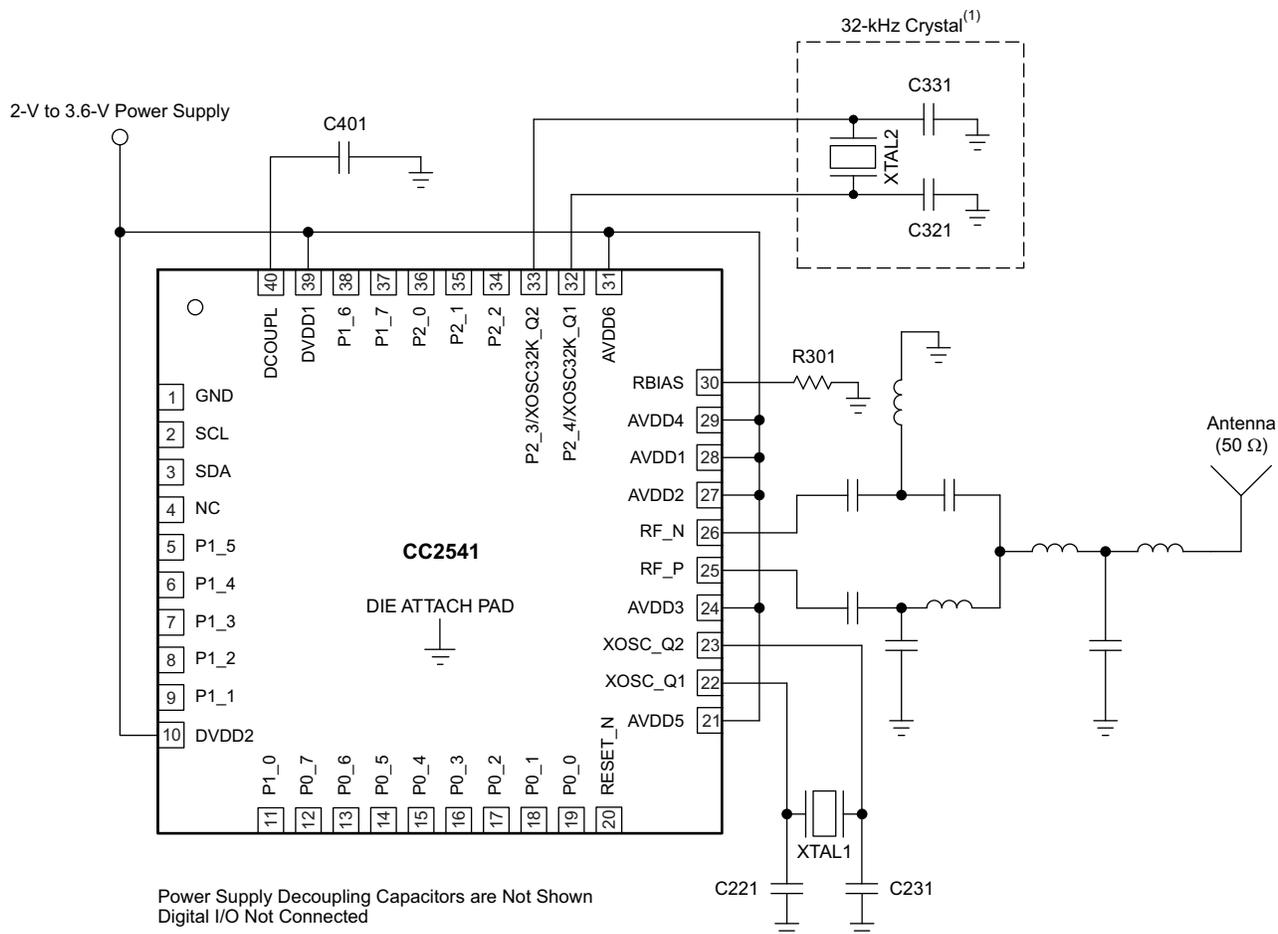
(1) 32-kHz crystal is mandatory when running the BLE protocol stack in low-power modes, except if the link layer is in the standby state (Vol. 6 Part B Section 1.1 in [1]).
