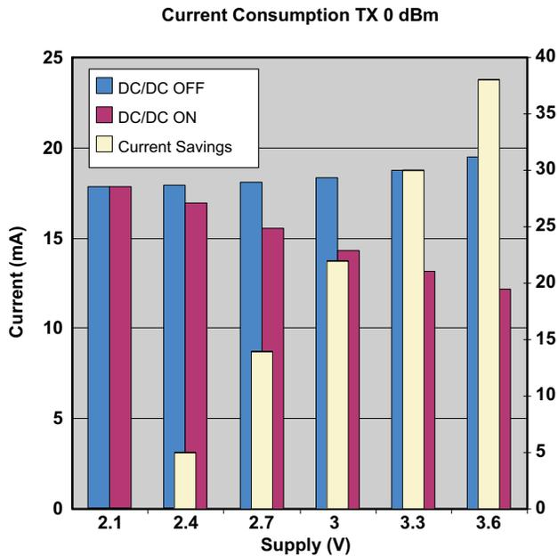
**Figure 20. Current Savings in TX at Room Temperature**
