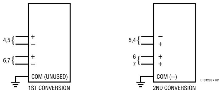
Figure 1. Examples of Multiplexer Options on the LTC1283
