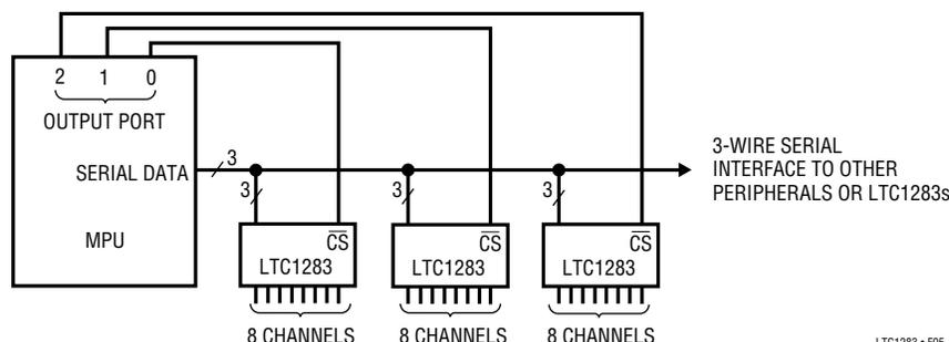
Figure 5. Several LTC1283s Sharing One 3-Wire Serial Interface
