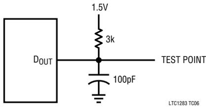
Voltage Waveform for D<sub>OUT</sub> Rise and Fall Times, t<sub>r</sub> and t<sub>f</sub>
