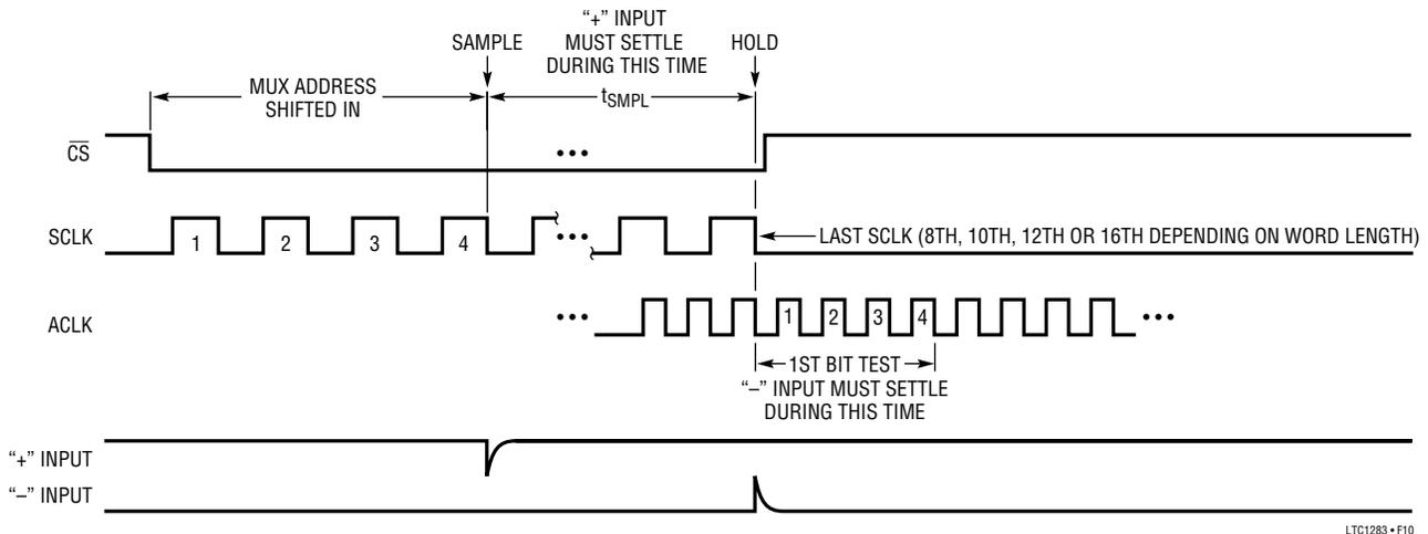
Figure 10. "+" and "-" Input Settling Windows
