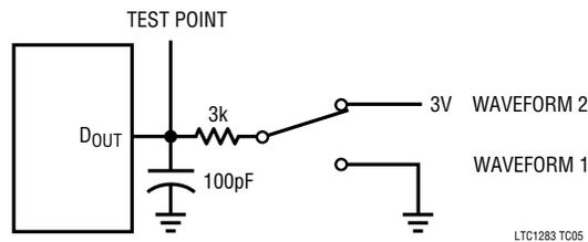
Voltage Waveforms for t<sub>en</sub> and t<sub>dis</sub>
