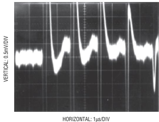
Figure 16. Poor Reference Settling Can Cause A/D Errors
