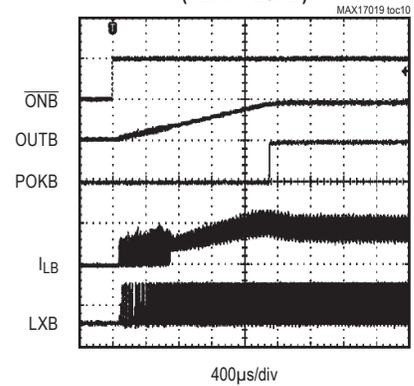
400 $\mu\text{s/div}$   $R_{LOAD} = 1.01\Omega$
