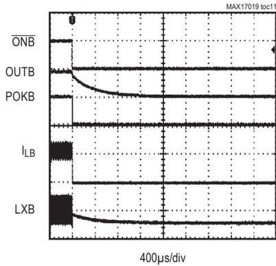
400 $\mu\text{s/div}$   $R_{LOAD} = 0.8\Omega$
