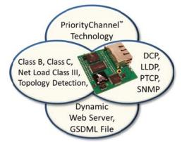
PROFINET support includes the Precision Time Control Protocol (PTCP) for synchronization of nodes in a network and the Discovery and
