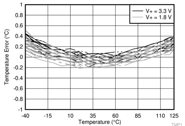
**Figure 6-5. Temperature Error vs. Temperature (YFF Package)**
