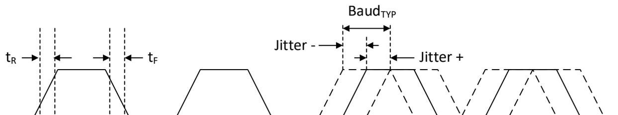
**Figure 6-1. SMART Wire™ / UART Interface Timing Diagram**
