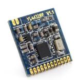
433MHz wireless ISM transceiver module
