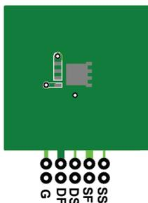
50  $^\circ\text{C/W}$  when mounted on a  $1\text{ in}^2$  pad of 2 oz copper
