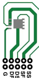
125  $^\circ\text{C/W}$  when mounted on a minimum pad of 2 oz copper.
