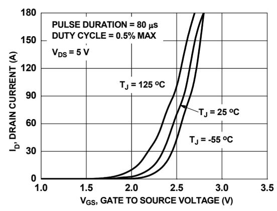
Figure 5. Transfer Characteristics
