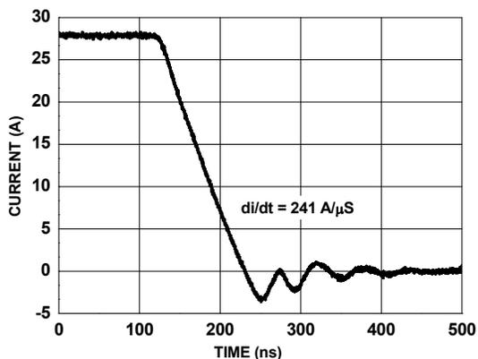
Figure 14. FDMS2D4N03S SyncFET<sup>™</sup> Body Diode Reverse Recovery Characteristic
