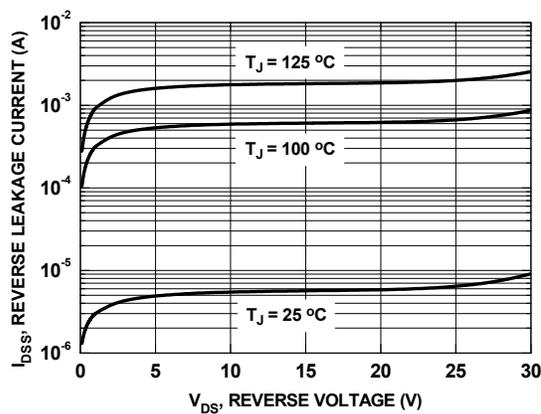
Figure 15. SyncFET<sup>™</sup> Body Diode Reverse Leakage vs. Drain-Source Voltage
