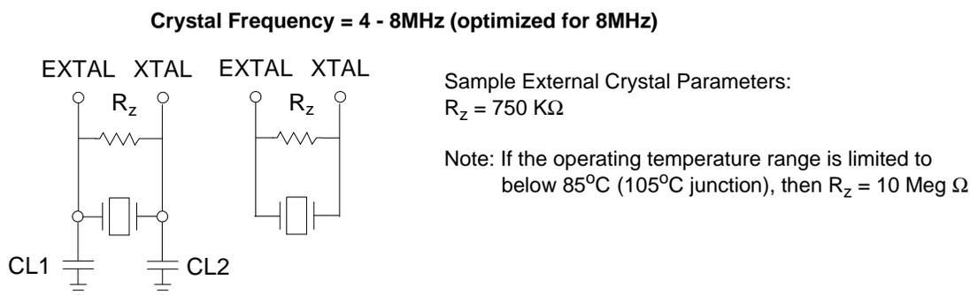
**Figure 3-1 External Crystal Oscillator Circuit**
