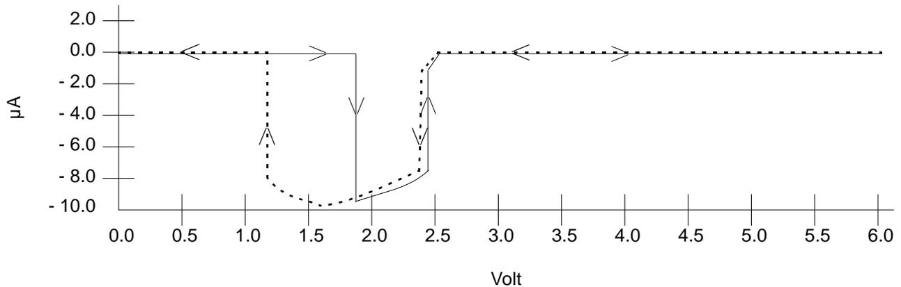
**Figure 10-1  $I_{IN}/I_{OZ}$  vs.  $V_{IN}$  (Typical; Pull-Up Disabled)**
