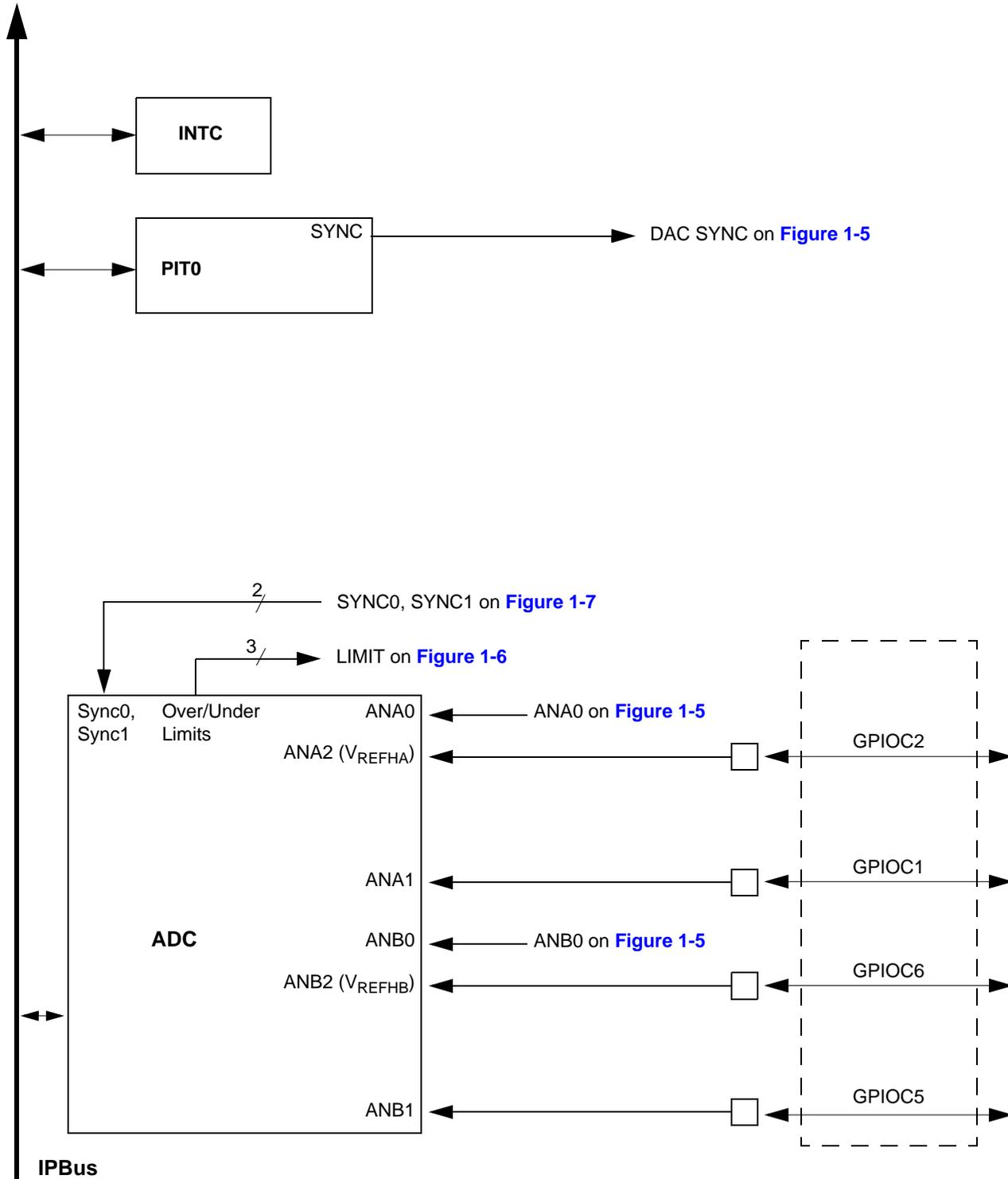
Figure 1-3 56F8033/56F8023 I/O Pin-Out Muxing (Part 1/5)
