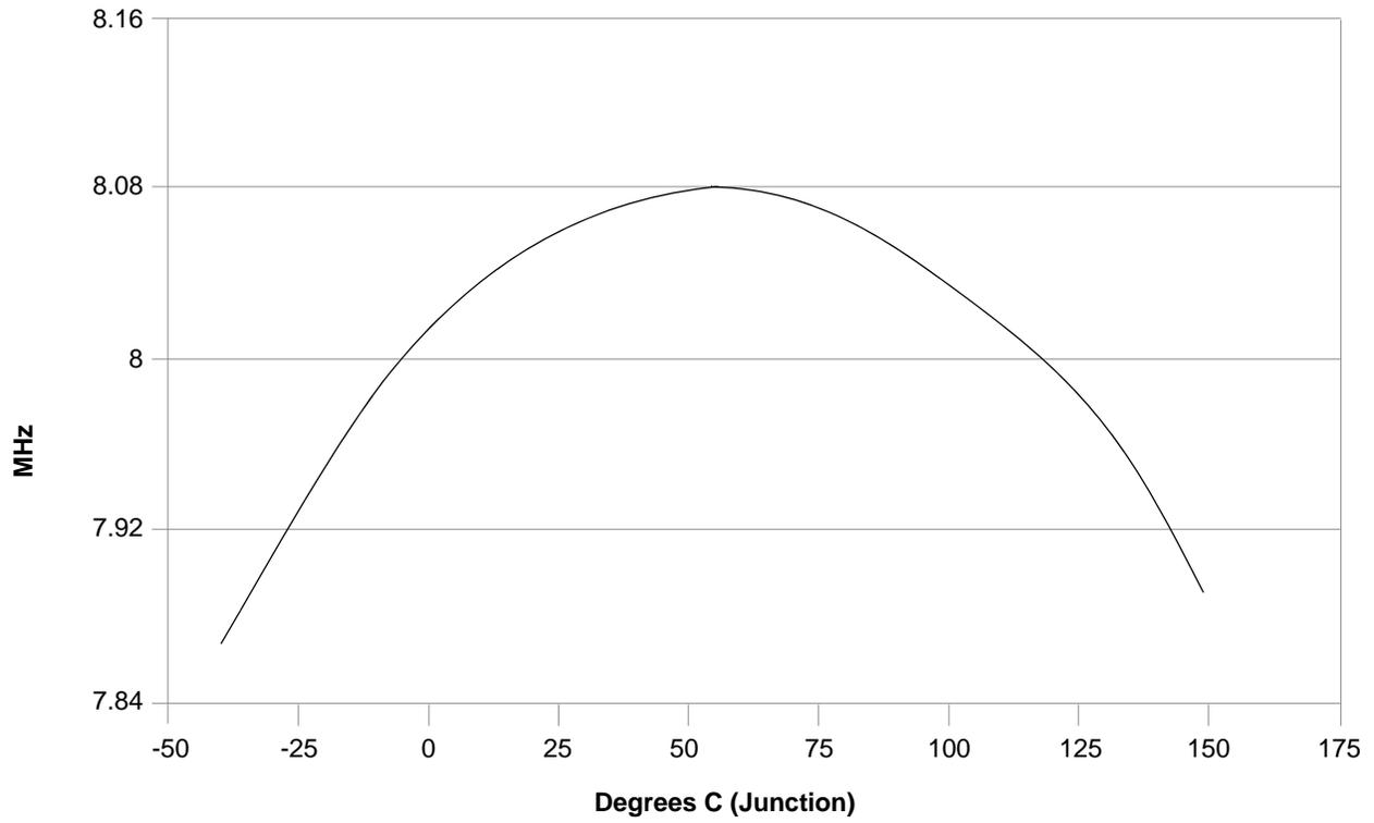
**Figure 10-5 Relaxation Oscillator Temperature Variation (Typical) After Trim**
