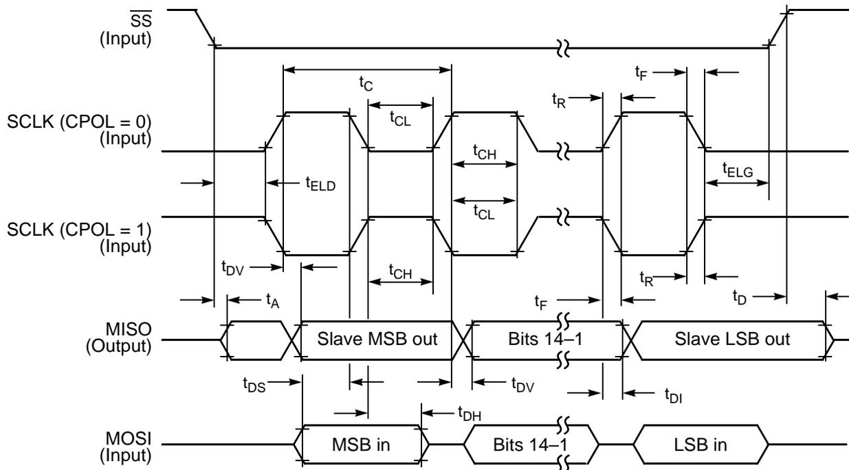
**Figure 10-10 SPI Slave Timing (CPHA = 1)**
