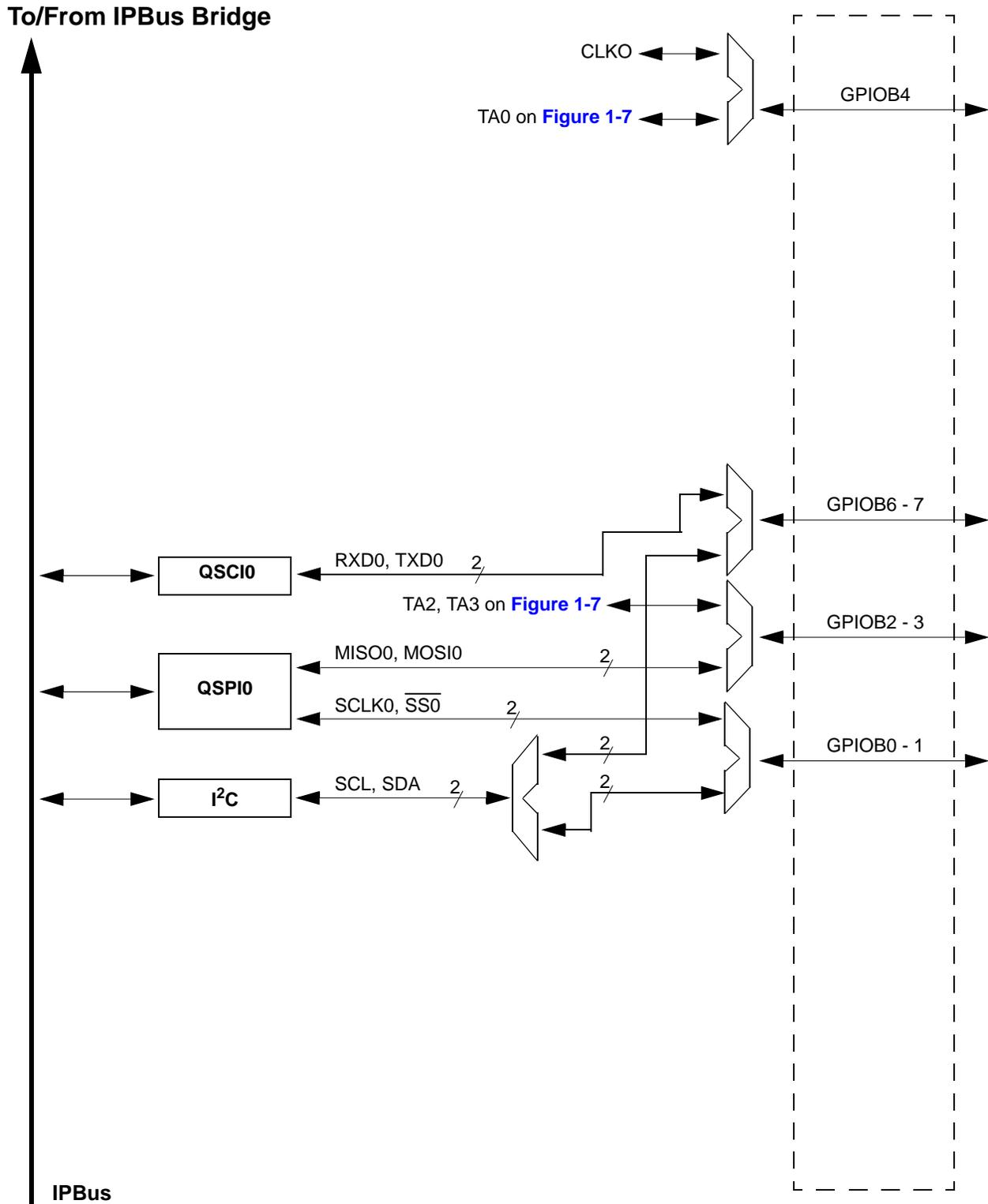
Figure 1-4 56F8033/56F8023 I/O Pin-Out Muxing (Part 2/5)
