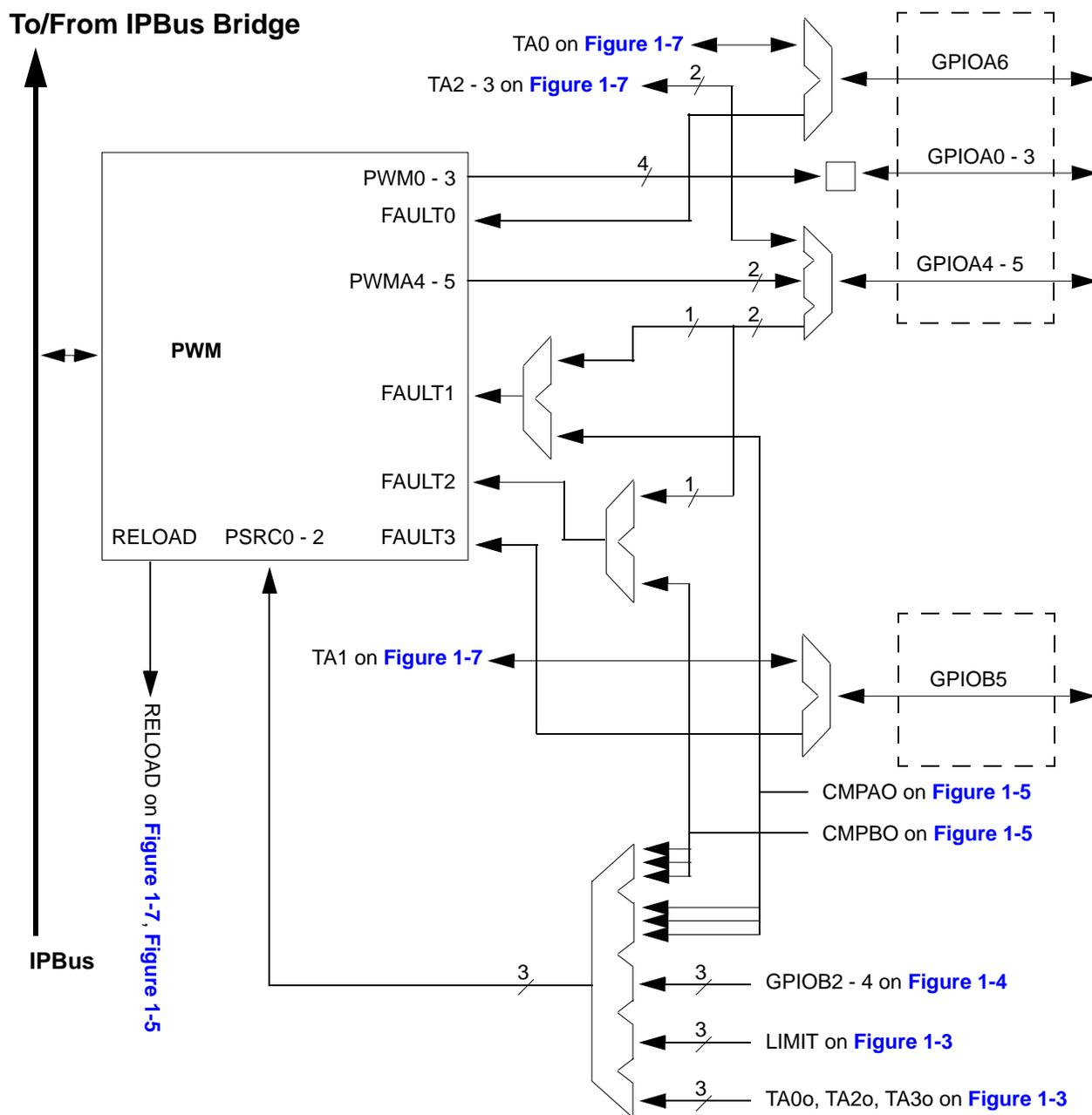
Figure 1-6 56F8033/56F8023 I/O Pin-Out Muxing (Part 4/5)
