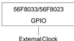
**Figure 3-4 Connecting an External Clock Signal using GPIO**
