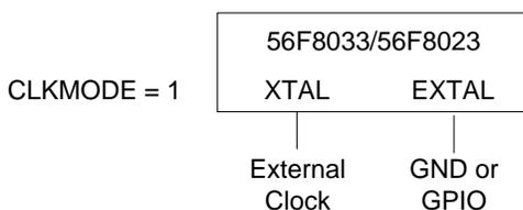
**Figure 3-3 Connecting an External Clock Signal using XTAL**
