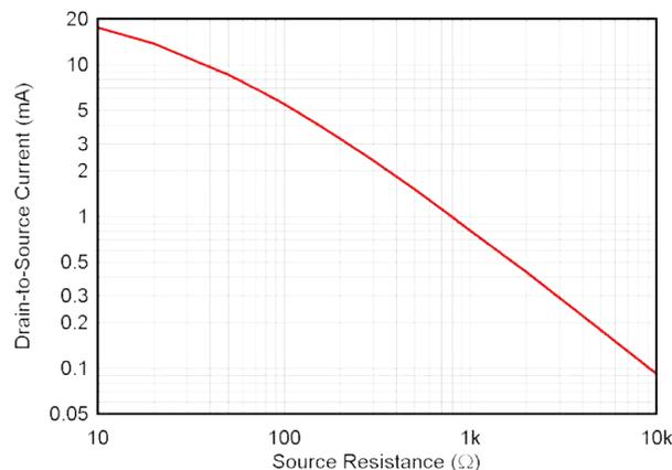
**Figure 9-3. Drain-to-Source Current vs  $R_S$ ,  $V_{DS} = 5 \text{ V}$**
