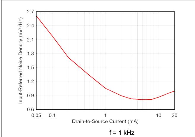
**Figure 6-11. Input-Referred Noise Spectral Density vs Drain-to-Source Current**
