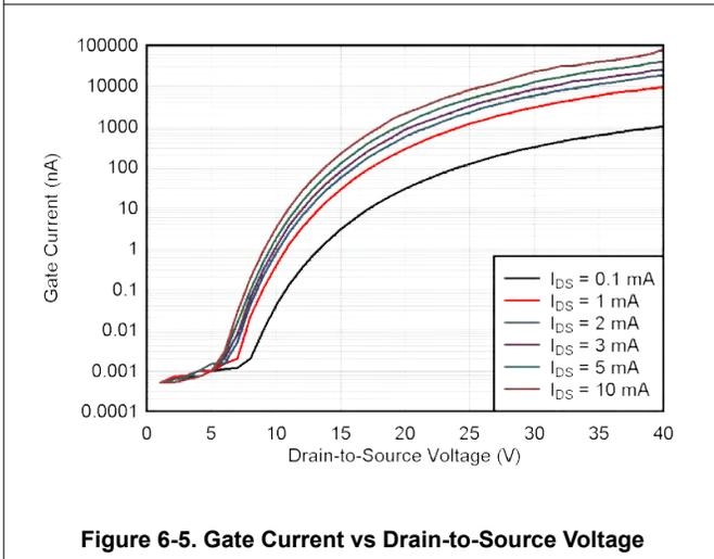
Figure 6-5. Gate Current vs Drain-to-Source Voltage
