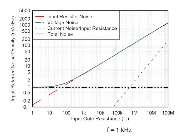
**Figure 6-10. Noise Density Contributors vs Input Gate Resistance**
