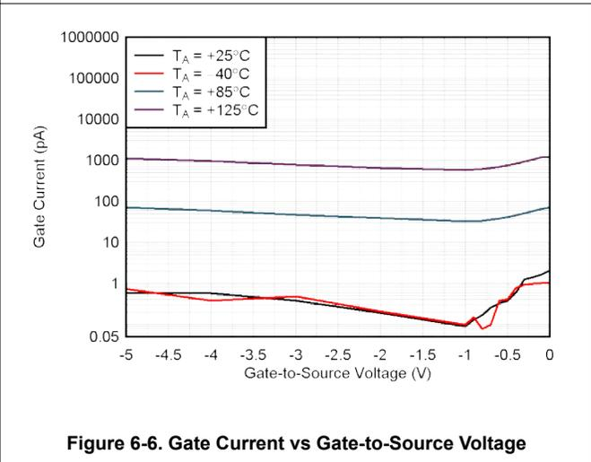
Figure 6-6. Gate Current vs Gate-to-Source Voltage
