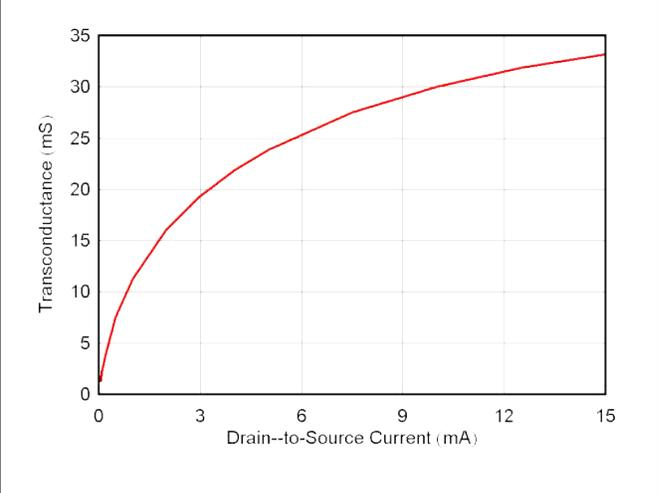
Figure 6-4. Common Source Transconductance vs Drain-to-Source Current
