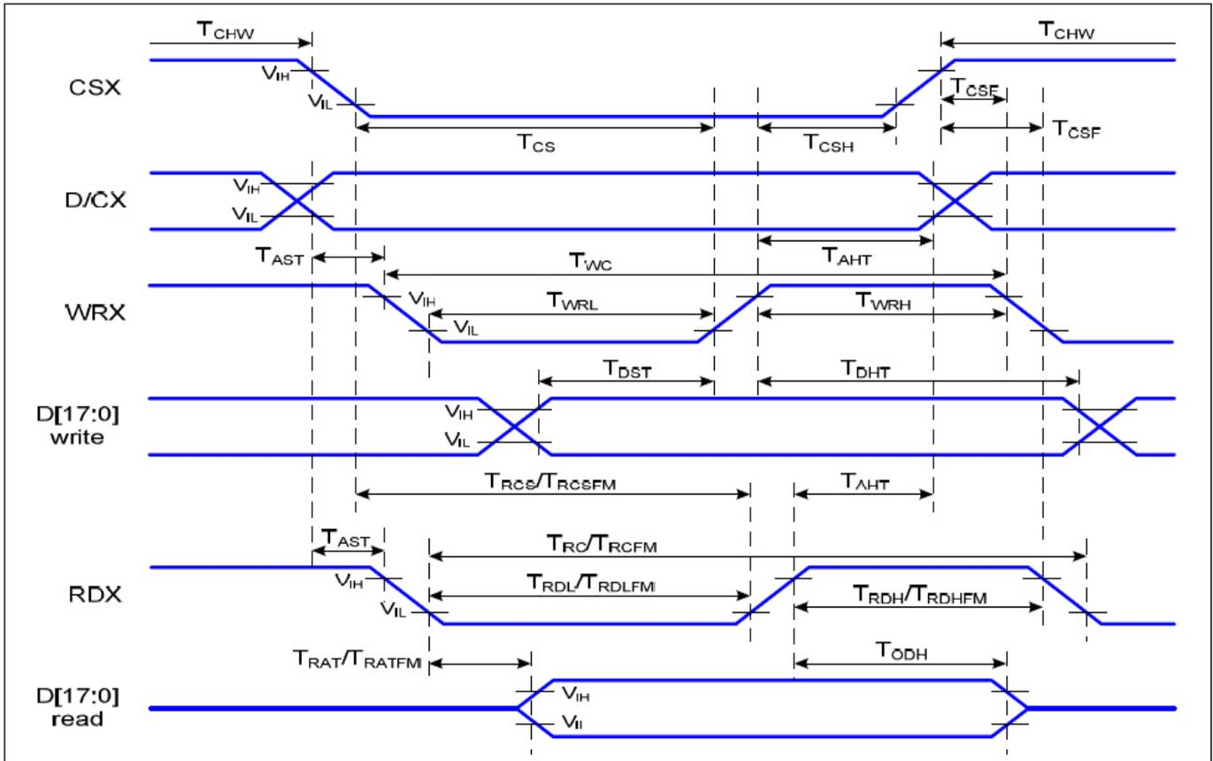
Figure 6.2: 8080 MCU Parallel Interface Timing Diagram
