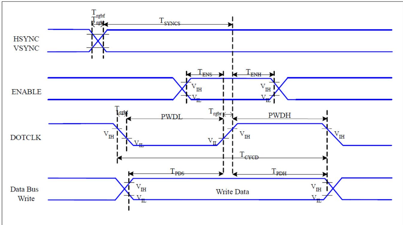
Figure 6.1: RGB Interface Timing Characteristics
