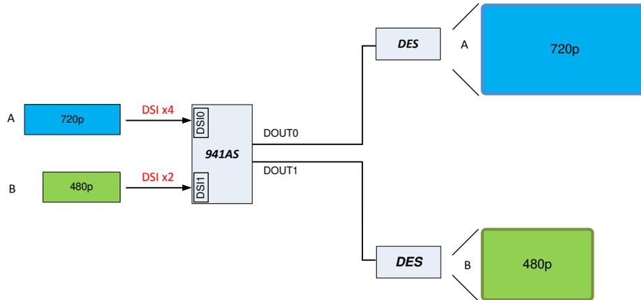
**Figure 8-17. Independent 2:2 Mode With DSI Reference Clock**
