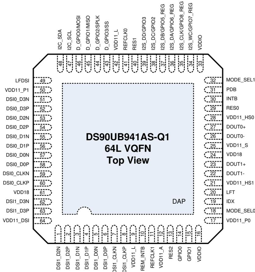
Figure 6-1. RTD Package 64-Pin VQFN Top View
