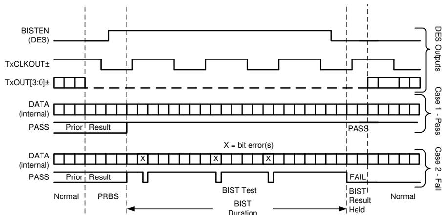
**Figure 8-11. BIST Waveforms in Conjunction With Deserializer Signals**
