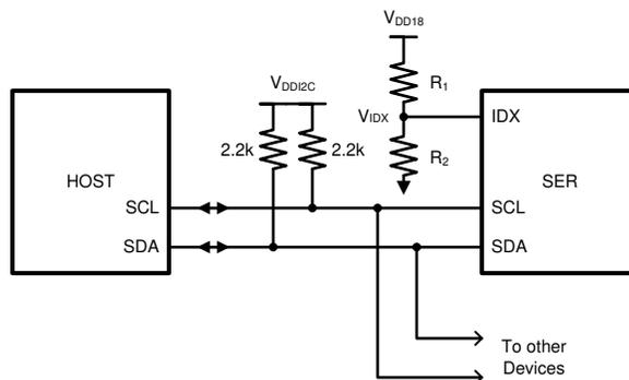
**Figure 8-29. Serial Control Bus Connection**
