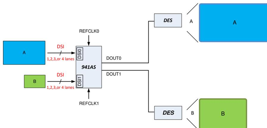
**Figure 8-18. Independent 2:2 Mode With External Reference Clocks**
