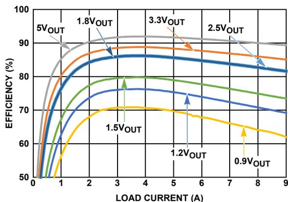
FIGURE 6. EFFICIENCY vs LOAD, VIN = 12V, 300kHz
