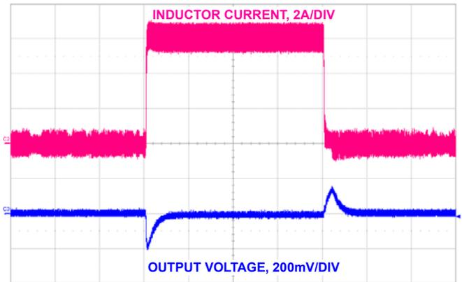
FIGURE 39. 6A LOAD TRANSIENT RESPONSE, DIODE EMULATION
