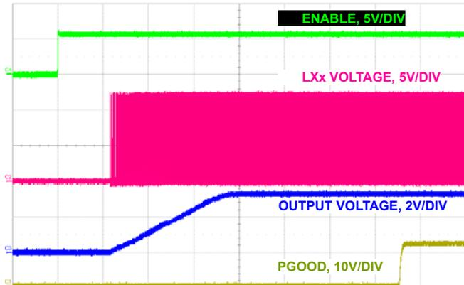
FIGURE 32. MONOTONIC SOFT-START WITH NO LOAD, CCM
