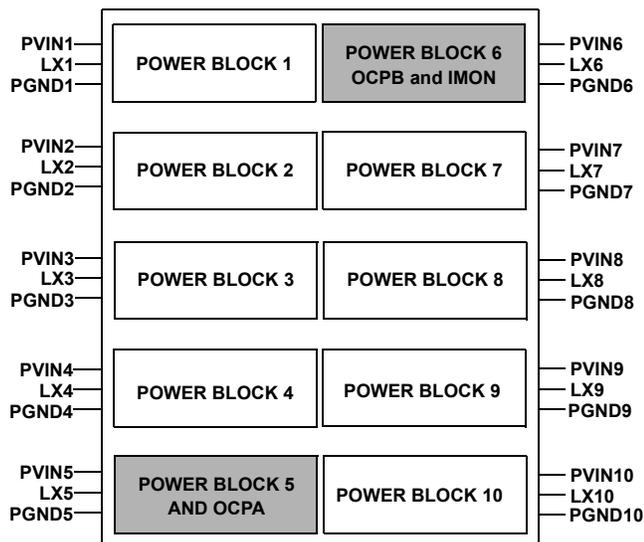
Note: Shaded blocks indicate pilot current and current sensors.
