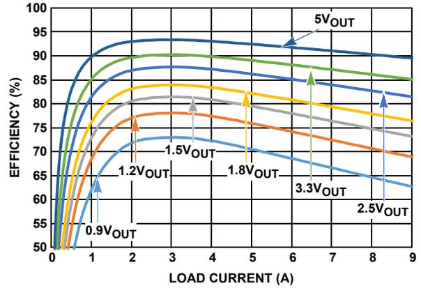
FIGURE 9. EFFICIENCY vs LOAD,  $V_{IN} = 8V$ , 500kHz
