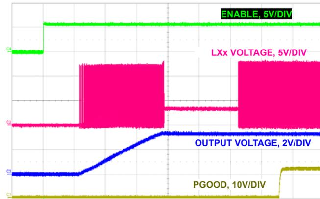
FIGURE 35. MONOTONIC SOFT-START WITH NO LOAD, DEM
