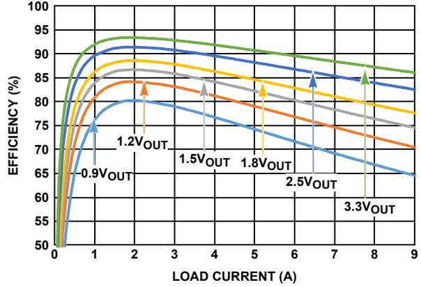
FIGURE 11. EFFICIENCY vs LOAD,  $V_{IN} = 5V$ , 500kHz
