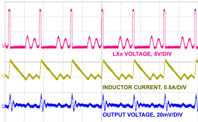
FIGURE 38. DIODE EMULATION OPERATION,  $V_{OUT} = 1.2V$ , 125mA LOAD
