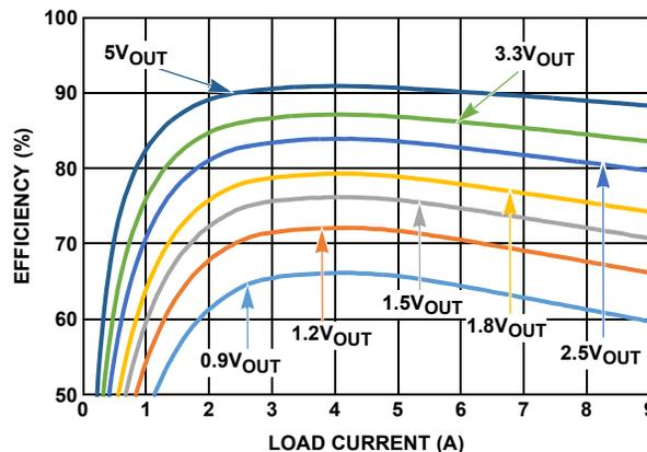
FIGURE 7. EFFICIENCY vs LOAD, VIN = 12V, 500kHz
