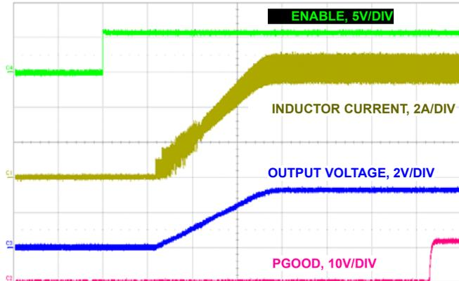
FIGURE 33. MONOTONIC SOFT-START WITH 6A LOAD, CCM
