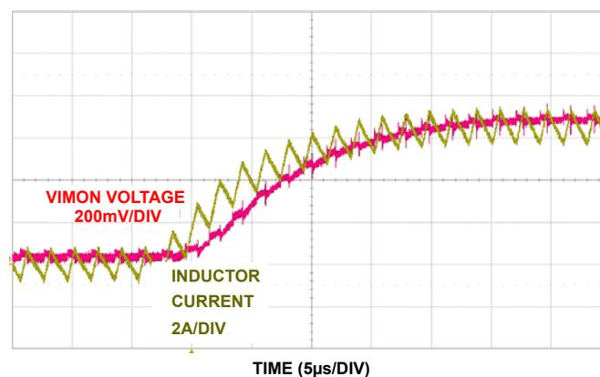
**FIGURE 51. IMON RESPONSE TO 6A LOAD STEP**
