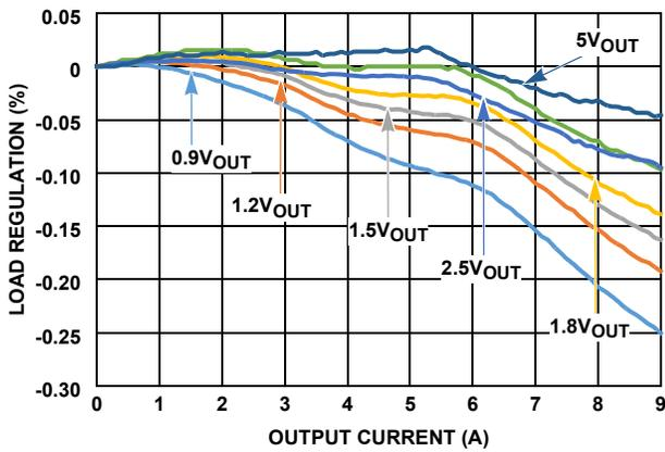
FIGURE 24. LOAD REGULATION vs  $V_{OUT}$ ,  $PV_{IN} = 12V$
