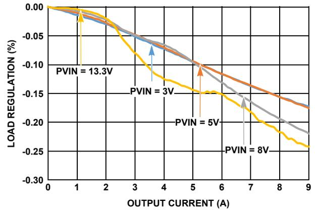
FIGURE 25. LOAD REGULATION vs  $PV_{IN}$ ,  $V_{OUT} = 1.0V$
