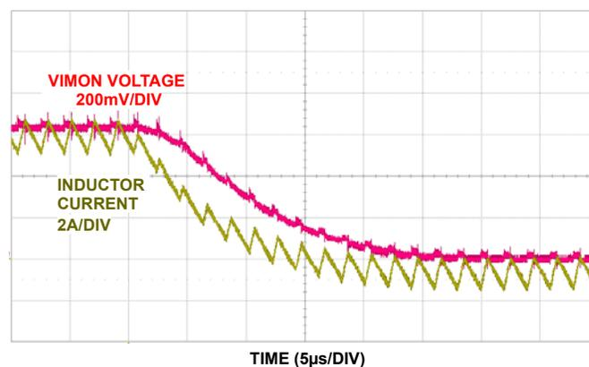
**FIGURE 52. IMON RESPONSE TO 6A LOAD RELEASE**
