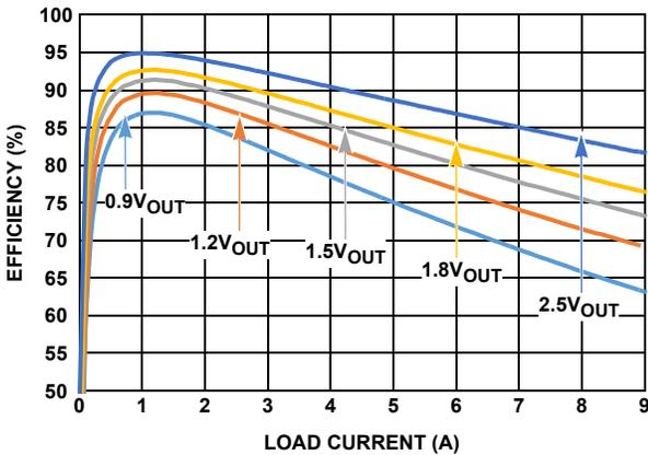
FIGURE 12. EFFICIENCY vs LOAD,  $V_{IN} = 3.3V$ , 300kHz
