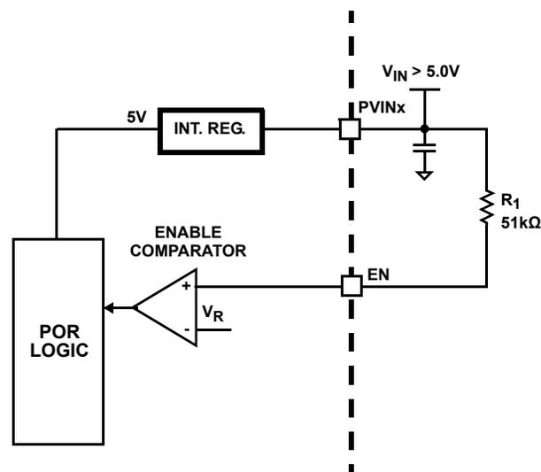
FIGURE 45. ENABLE TO  $V_{IN}$  FOR >5.0V INPUT VOLTAGE
