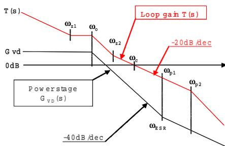
Figure 8. Asymptotic diagram of buck power stage and its compensated loop gain.
