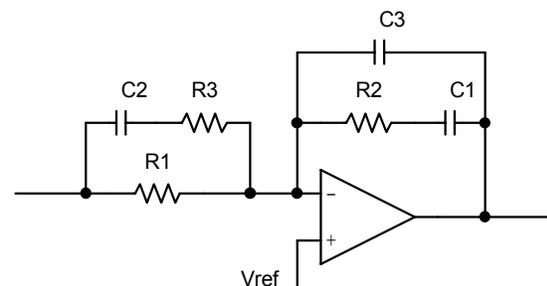
Figure 7. Voltage Mode Buck Converter Compensation Network
