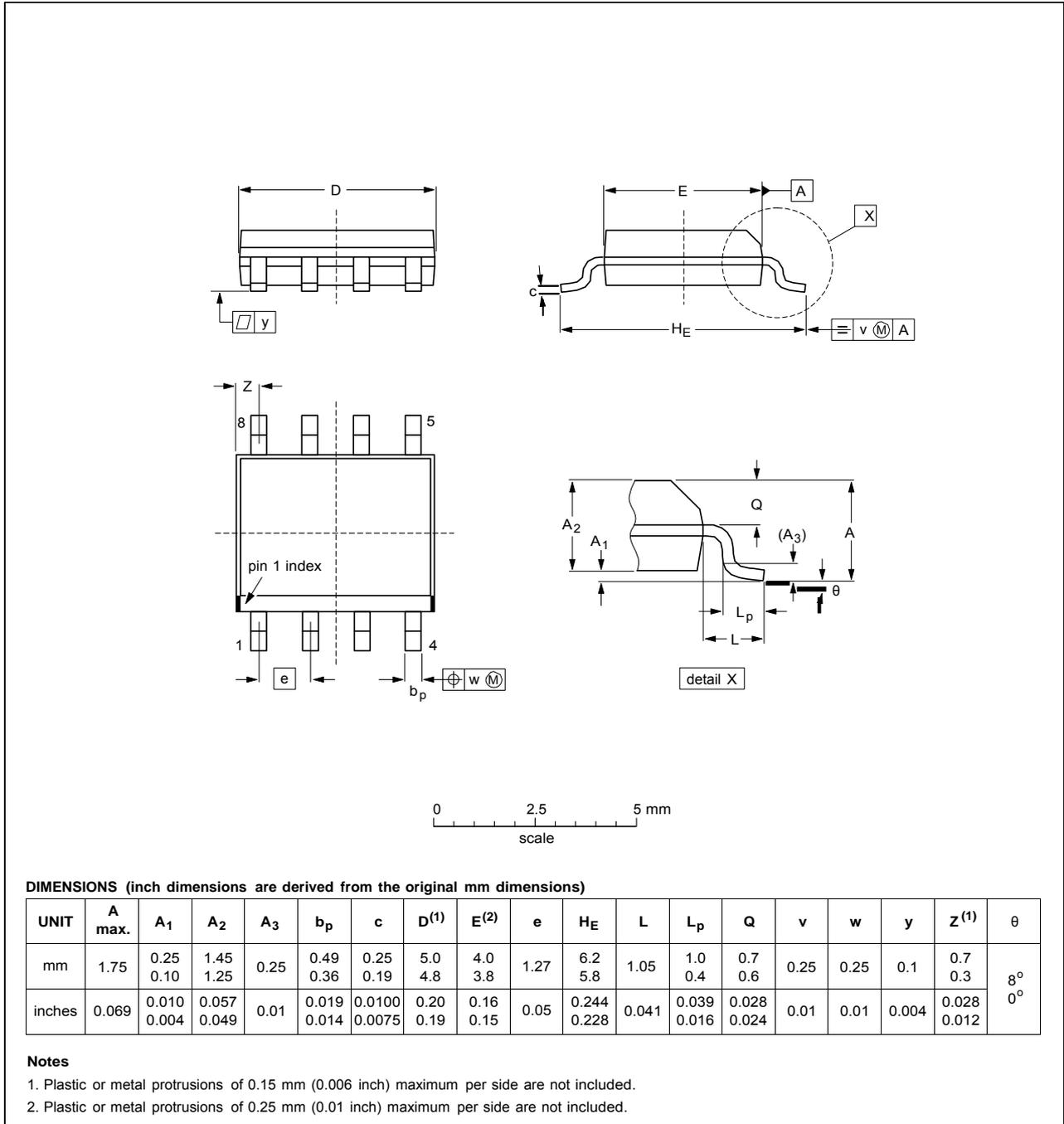
MSOP8: plastic thin shrink small outline package; 8 leads; body width 3 mm
