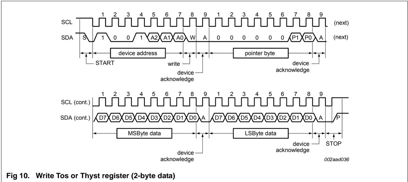
Fig 10. Write Tos or Thyst register (2-byte data)
