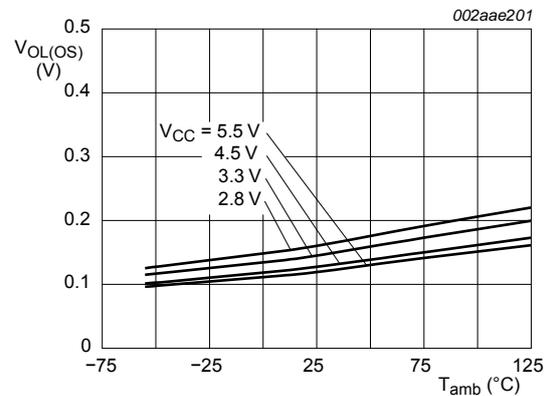
**Fig 17. LOW-level output voltage on pin OS versus temperature; I<sub>OL</sub> = 4 mA**
