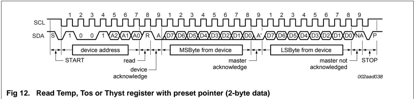
Fig 12. Read Temp, Tos or Thyst register with preset pointer (2-byte data)
