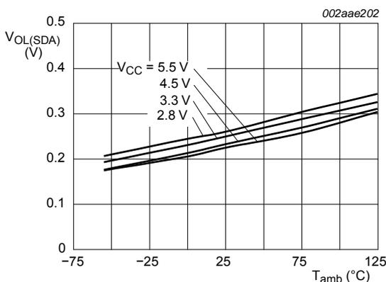
**Fig 18. LOW-level output voltage on pin SDA versus temperature; I<sub>OL</sub> = 4 mA**
