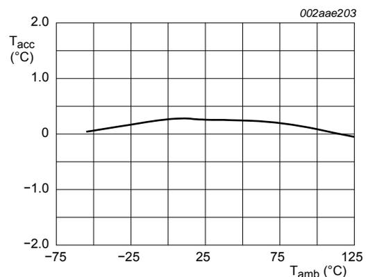
**Fig 19. Typical temperature accuracy versus temperature; V<sub>CC</sub> = 3.3 V**
