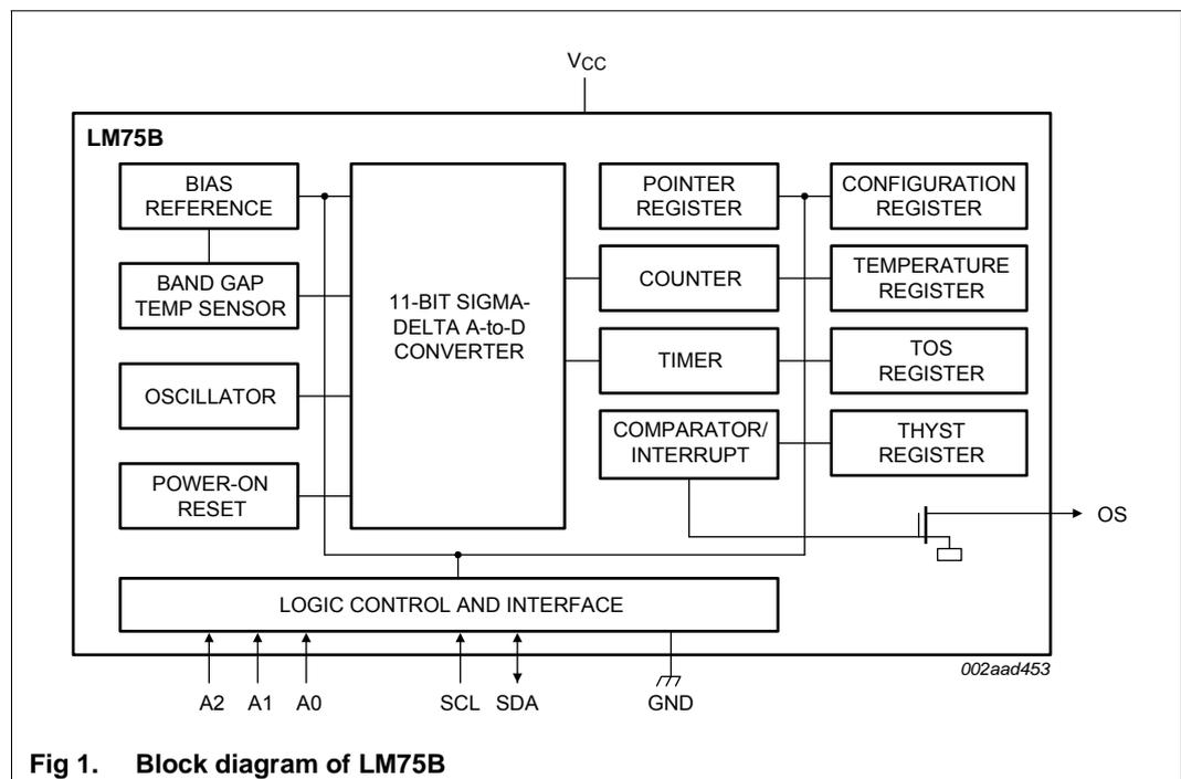
Fig 1. Block diagram of LM75B
