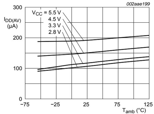
**Fig 15. Average supply current versus temperature; I<sup>2</sup>C-bus active**
