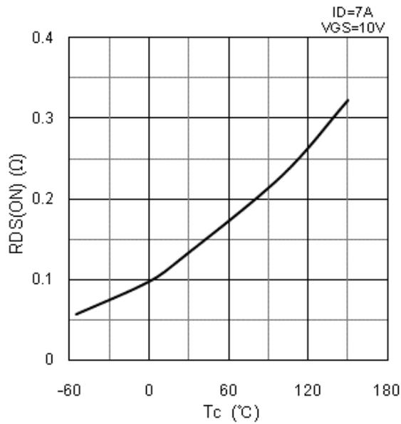
Figure 9.  $R_{DS(ON)}$  vs.  $T_c$
