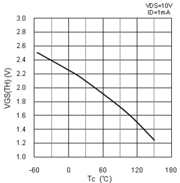
Figure 14.  $V_{GS(TH)}$  vs.  $T_c$
