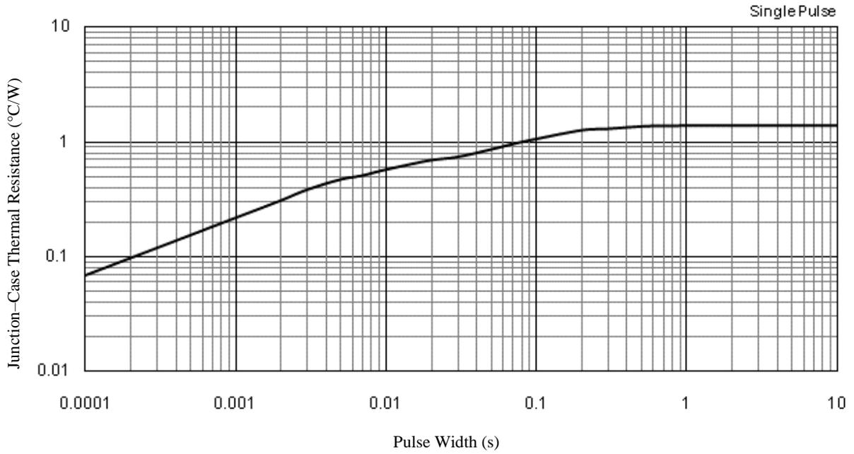
Figure 15. Transient Thermal Resistance Characteristics
