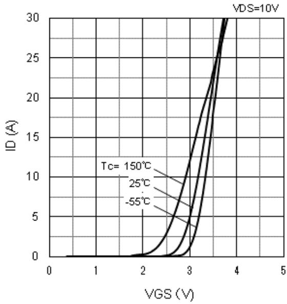
Figure 7.  $I_D$  vs.  $V_{GS}$
