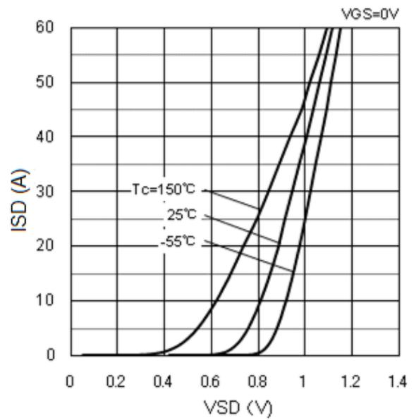
Figure 12.  $I_{SD}$  vs.  $V_{SD}$
