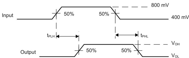
Figure 8. Propagation Delay
