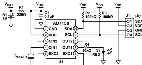
Figure 1. **AD7150** as a Proximity Detector in Standalone Operation
