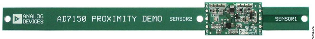
Figure 6. [AD7150](#) Door Handle Demonstration Board
