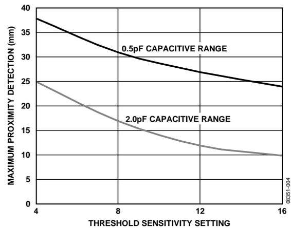
Figure 4. Typical Proximity Performance, Sensor 1
