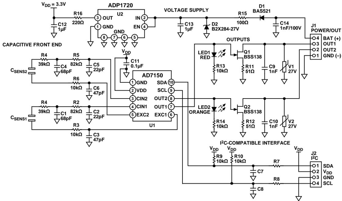
Figure 3. AD7150 in an Automotive Door Handle Application in Standalone Operation
