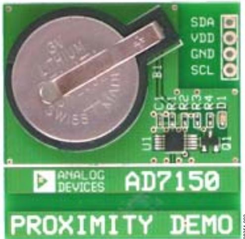
Figure 2. [AD7150](#) Proximity Detector Demonstration Board
