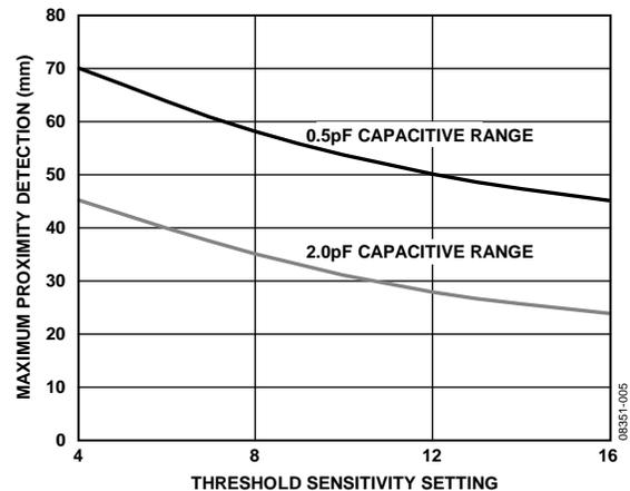
Figure 5. Typical Proximity Performance, Sensor 2
