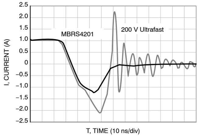
ON Semiconductor MBRS4201 eliminates reverse recovery oscillations present in Ultrafast devices in the market, particularly at hot temperatures.
