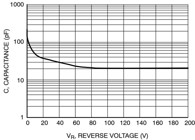
Figure 5. Typical Capacitance
