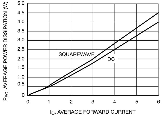
Figure 7. Power Dissipation
