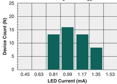
Typical  $I_F$  for Switch Dropout
