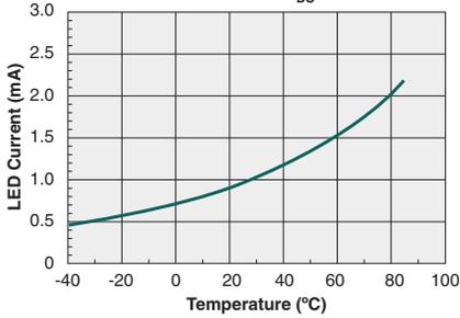
Typical  $I_F$  for Switch Dropout vs. Temperature
