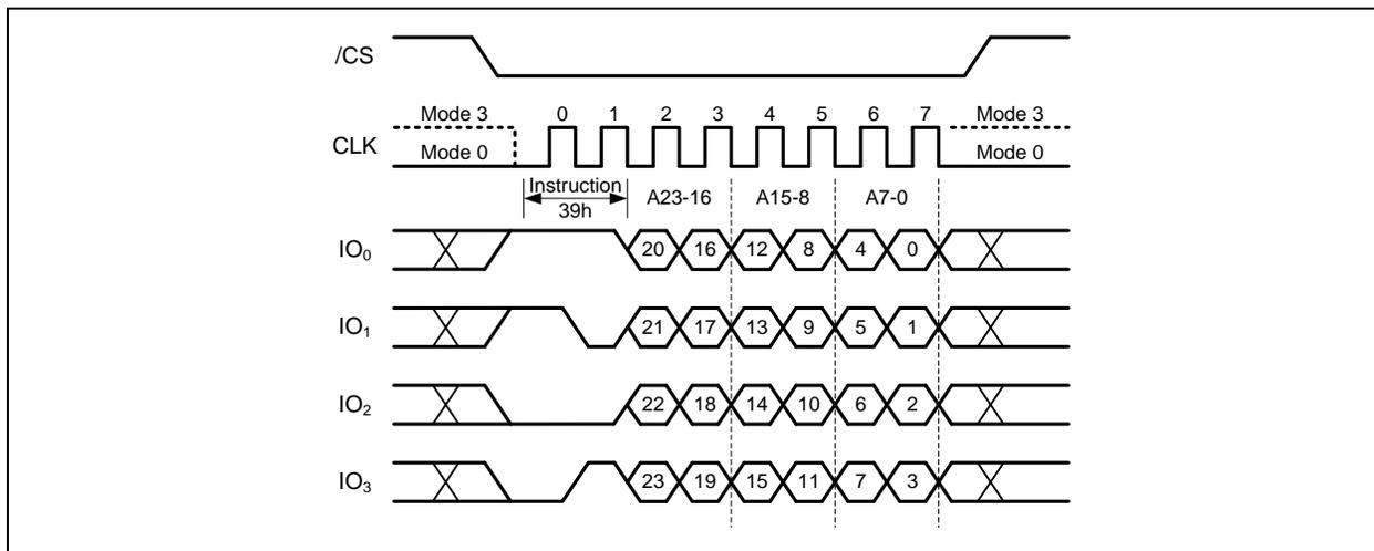
Figure 54b. Individual Block Unlock Instruction (QPI Mode)
