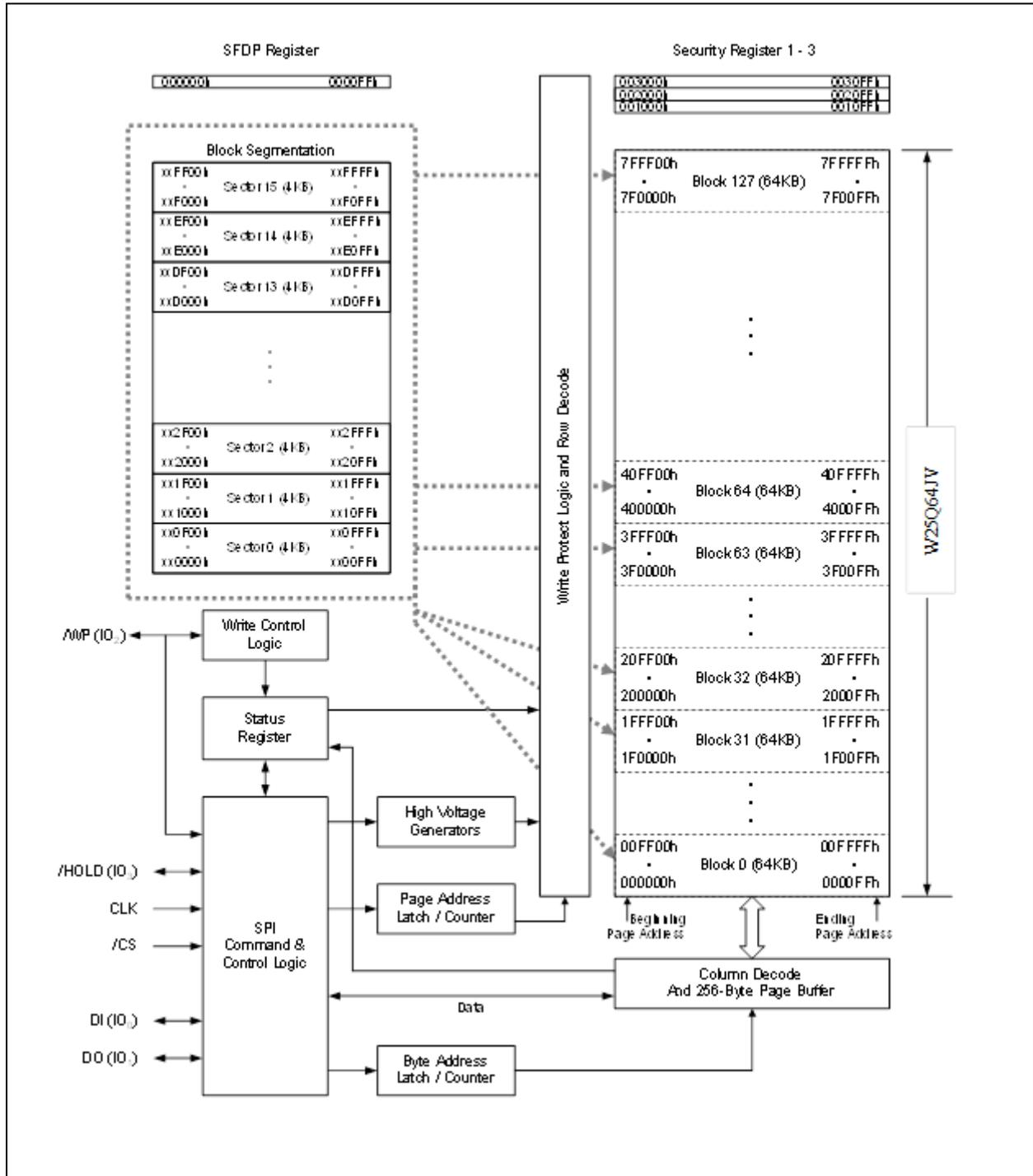
Figure 2. W25Q64JV Serial Flash Memory Block Diagram
