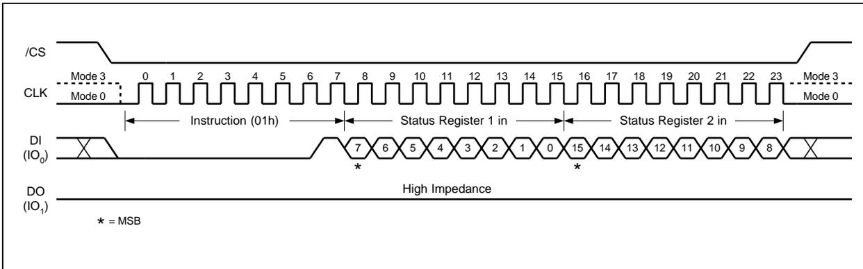
Figure 9c. Write Status Register-1/2 Instruction (SPI Mode)
