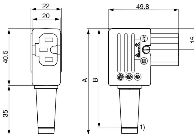
1) Cut strain relief 8 (10) mm here for 10 mm cable
