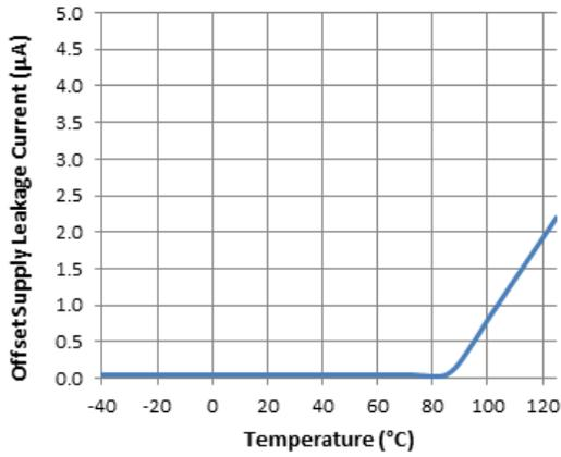
**Figure 28.** Offset Supply Leakage Current vs. Temperature
