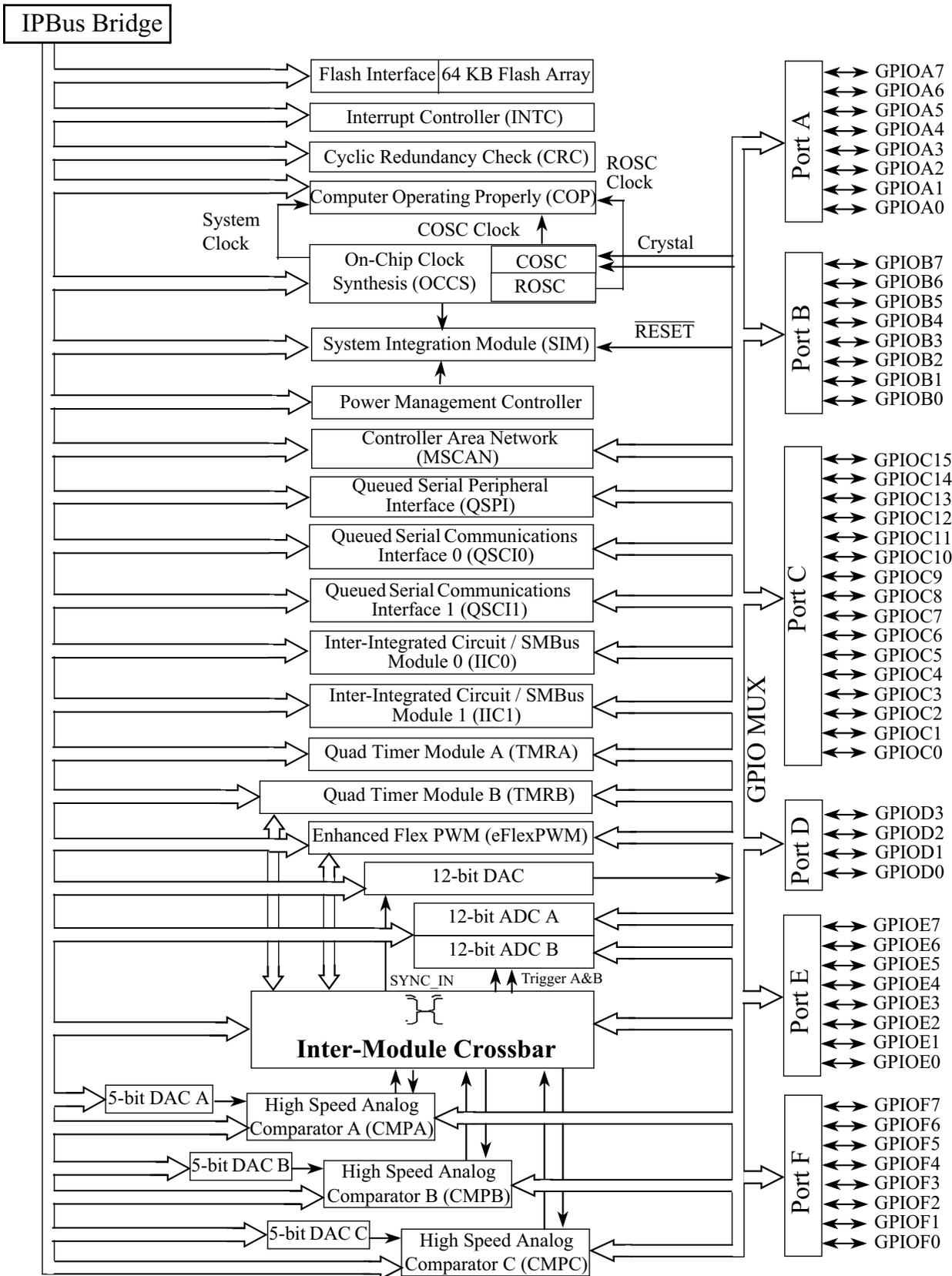
Figure 2. Peripheral Subsystem
