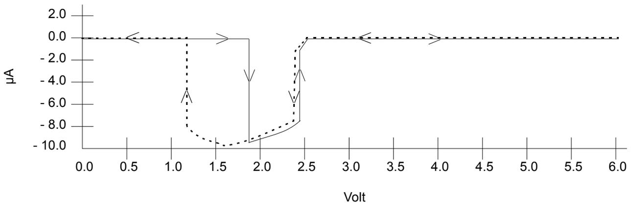
**Figure 14.  $I_{IN}/I_{OZ}$  versus  $V_{IN}$  (Typical; Pull-Up Disabled)**
