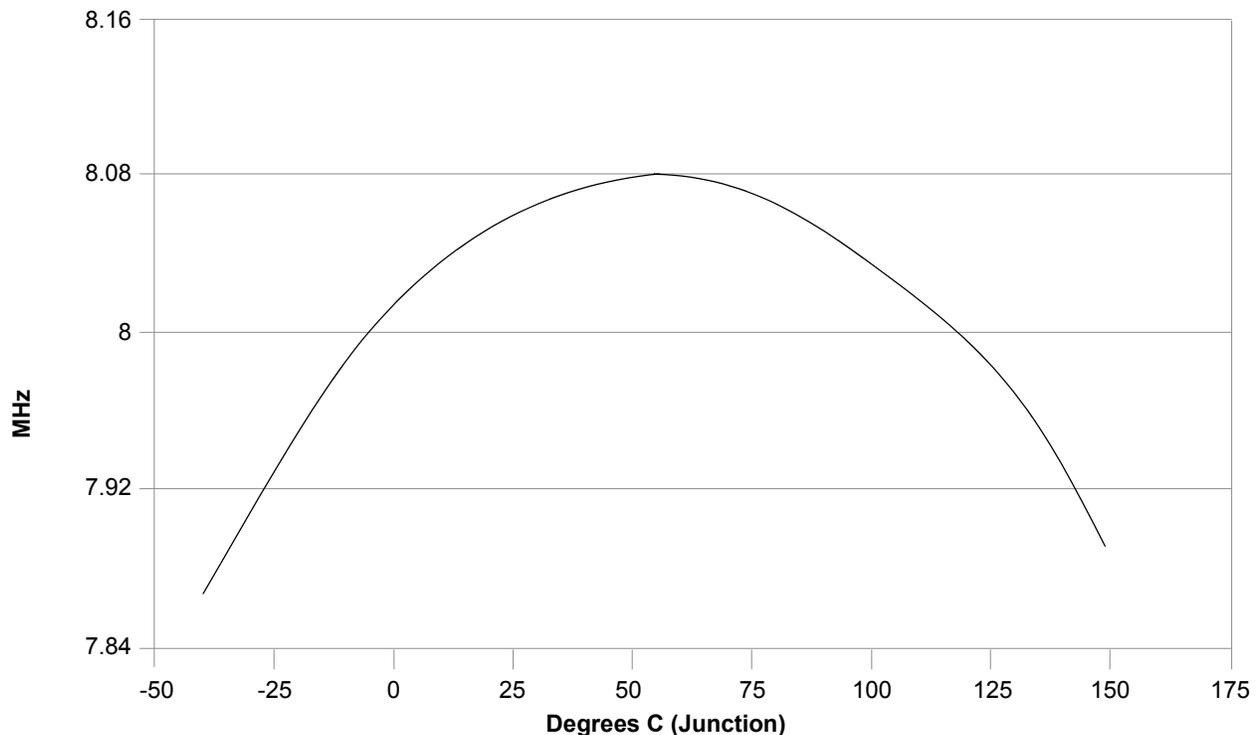
Figure 18. Relaxation Oscillator Temperature Variation (Typical) After Trim
