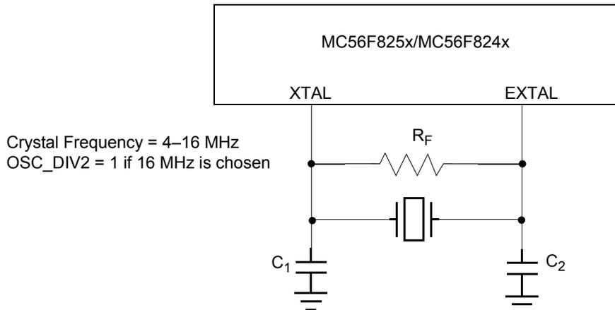
**Figure 10. Typical Crystal or Ceramic Resonator Circuit**
