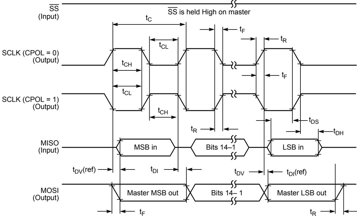
Figure 21. SPI Master Timing (CPHA = 1)
