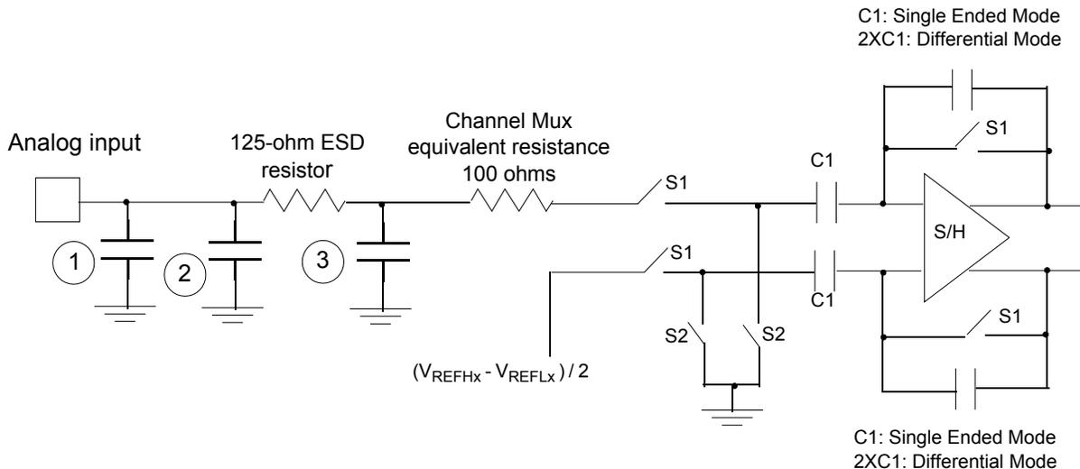
1. Parasitic capacitance due to package, pin-to-pin, and pin-to-package base coupling: 1.8 pF
