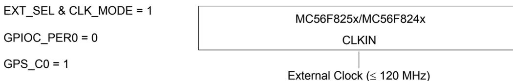
Figure 11. Connecting an External Clock Signal Using GPIO
