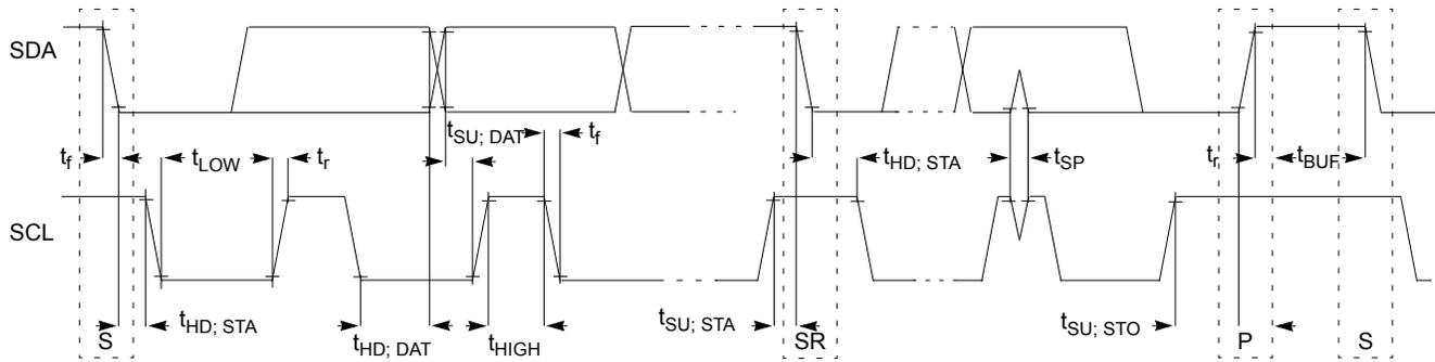
Figure 27. Timing Definition for Standard Mode Devices on the I<sup>2</sup>C Bus
