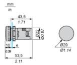
e Support panel thickness: 1 to 6 mm/0.4 to 0.24 in. (metal), 2 to 6 mm/0.8 to 0.24 in. (plastic).
