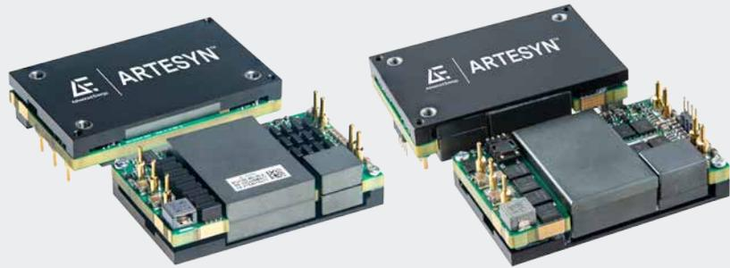
Advanced Energy's Artesyn BDQ1300 & BCQ1300 series quarter-brick are isolated DC-DC converters that produce a single 12V nominal output. Rated at 1300 watts, these converters can deliver up to 107 amps output current and has no minimum load requirement.
