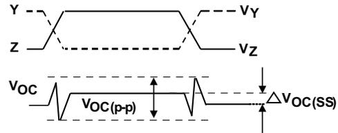
Input Generator PRR= 100 kHz, 50% duty cycle,  $t_r < 6\text{ ns}$ ,  $t_f < 6\text{ ns}$ ,  $Z_O = 50\Omega$
