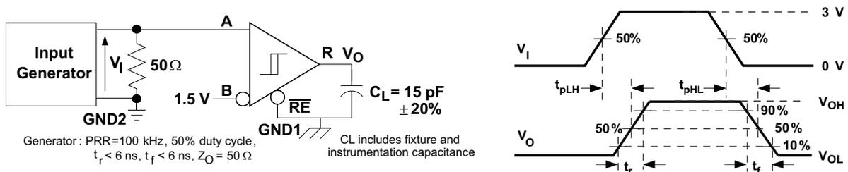
Figure 19. Receiver Switching Test Circuit and Waveforms
