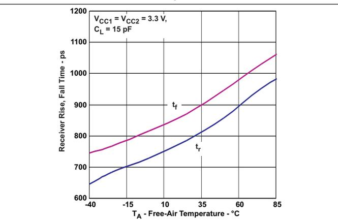
Figure 6. Receiver Rise, Fall Time vs Free-Air Temperature
