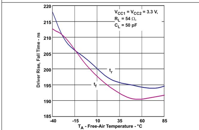
Figure 5. Driver Rise, Fall Time vs Free-Air Temperature
