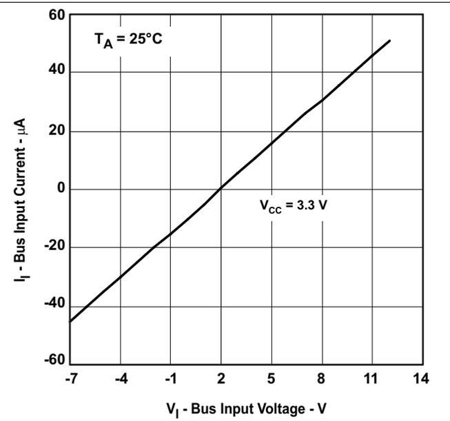
Figure 10. Bus Input Current vs Input Voltage
