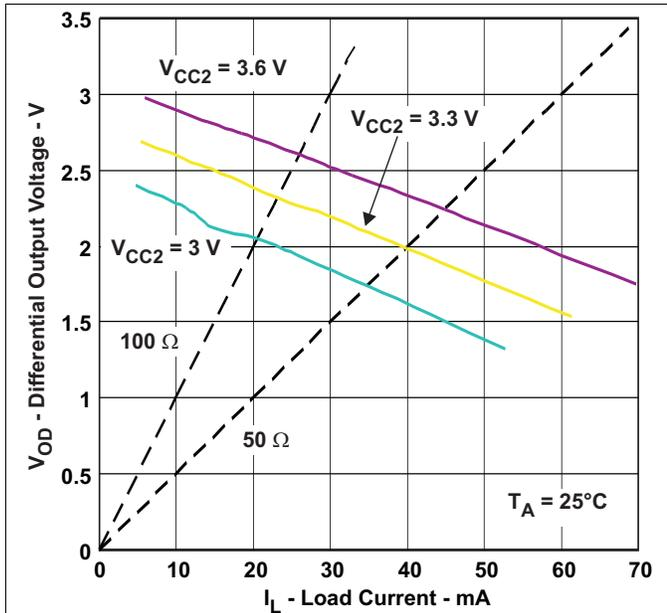
Figure 7. Differential Output Voltage vs Load Current
