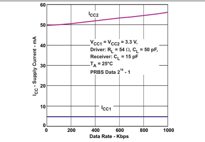
Figure 2. Supply Current vs Data Rate With Load
