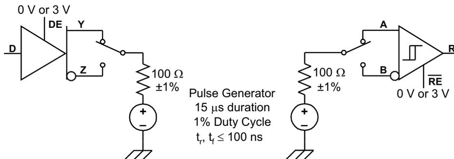
Figure 22. Transient Over-Voltage Test Circuit
