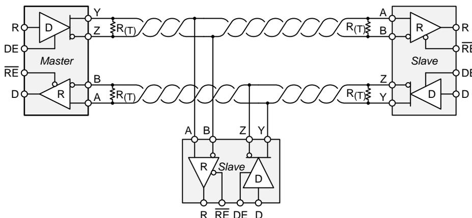
Figure 28. Typical RS-485 Network With Full-Duplex Transceivers
