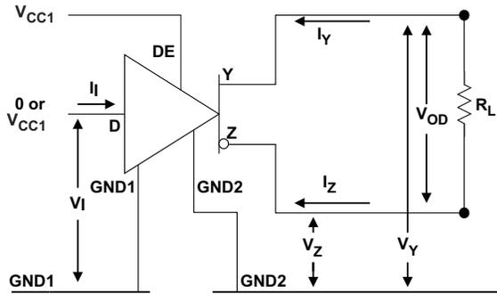
Figure 11. Driver  $V_{OD}$  Test and Current Definitions
