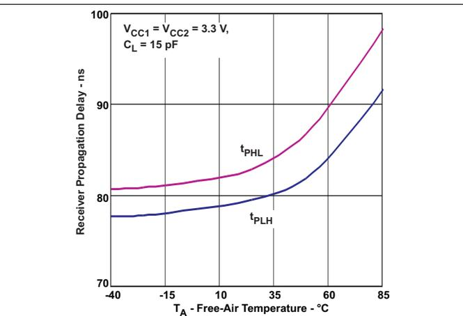
Figure 4. Receiver Propagation Delay vs Free-Air Temperature
