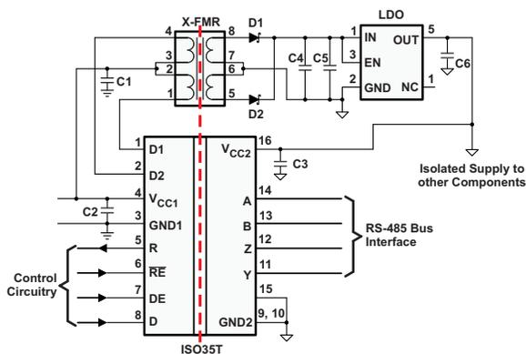
Figure 29. Typical Application Circuit
