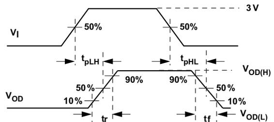
Figure 15. Driver Switching Test Circuit and Voltage Waveforms
