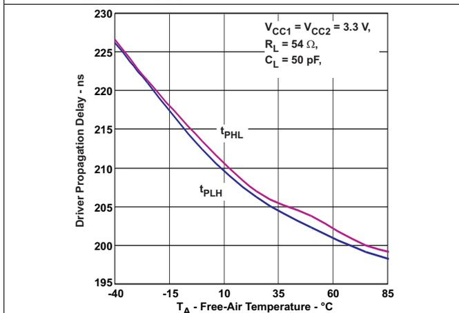
Figure 3. Driver Propagation Delay vs Free-Air Temperature
