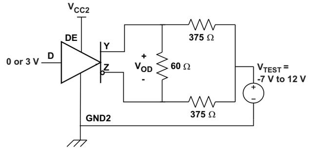
Figure 12. Driver  $V_{OD}$  With Common-Mode Loading Test Circuit
