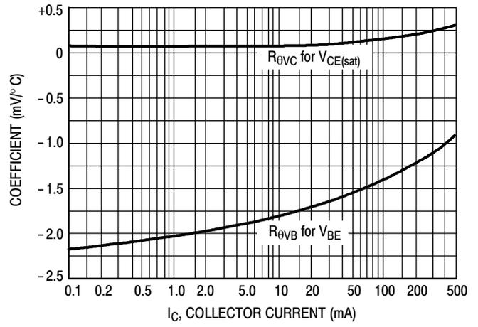
Figure 12. Temperature Coefficients
