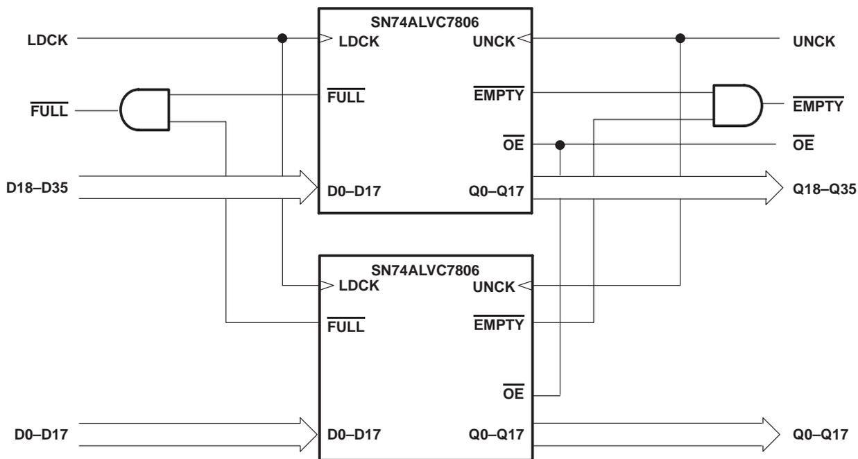
Figure 4. Word-Width Expansion: 256 × 36 Bits
